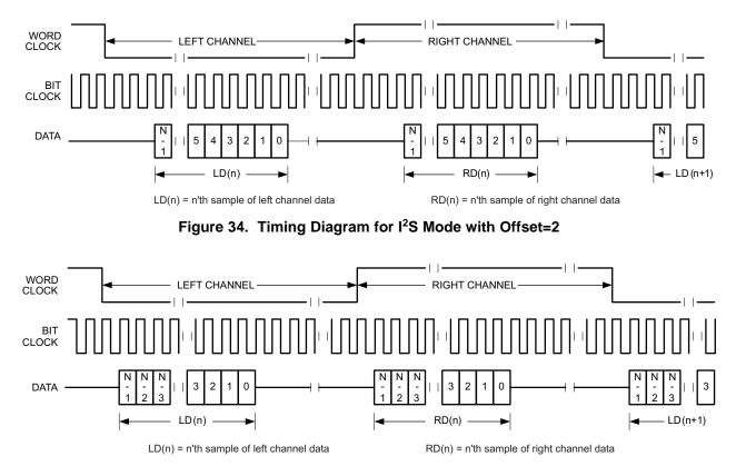
Figure 35. Timing Diagram for I<sup>2</sup>S Mode with Offset=0 and Inverted Bit Clock
