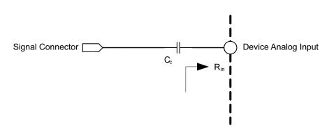
Figure 56. Analog Input Connection
