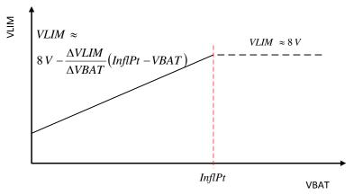
Figure 28. VLIM versus Supply Voltage (VBAT)
