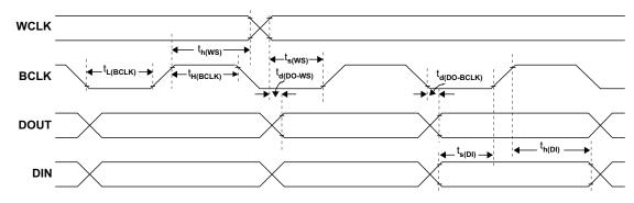
Figure 37. I<sup>2</sup>S/LJF/RJF Timing in Slave Mode
