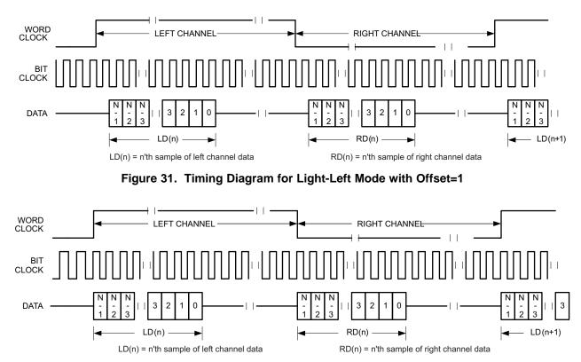
Figure 32. Timing Diagram for Left-Justified Mode with Offset=0 and Inverted Bit Clock
