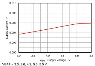
Figure 11. VBAT Quiescent Supply Current vs Supply Voltage
