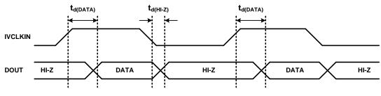
Figure 48. DOUT Timing in PDM Mode (Data on IVCLKIN High)
