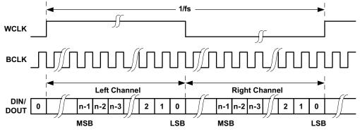
Figure 29. Timing Diagram for Right-Justified Mode
