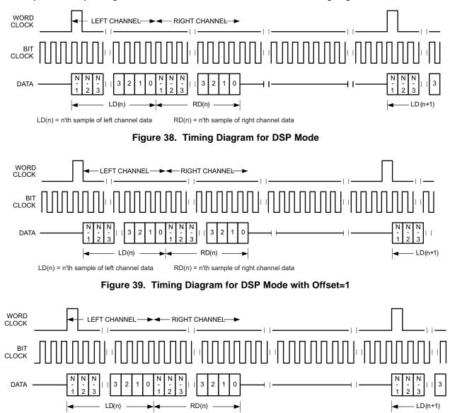
Figure 40. Timing Diagram for DSP Mode with Offset=0 and Inverted Bit Clock
