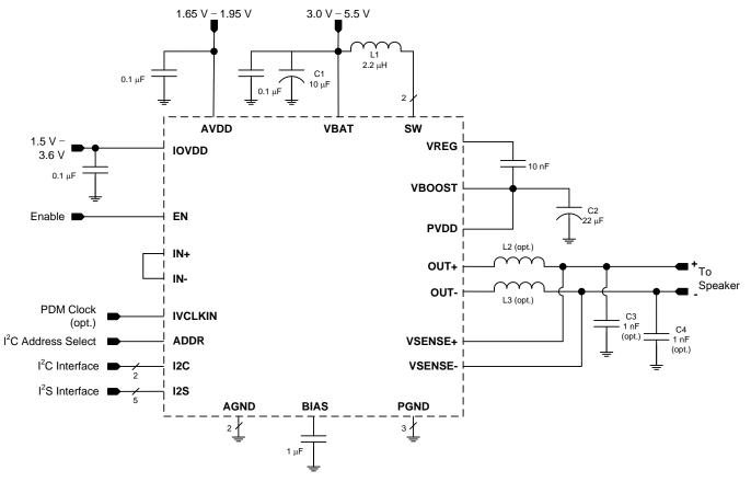
Figure 50. Typical Application Schematic
