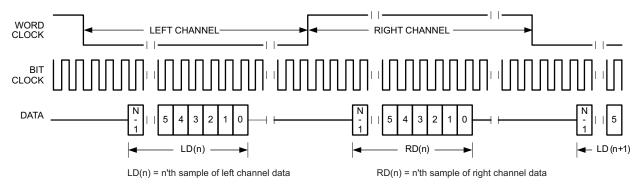
Figure 43. Timing Diagram for I<sup>2</sup>S in TDM Mode with Offset=2
