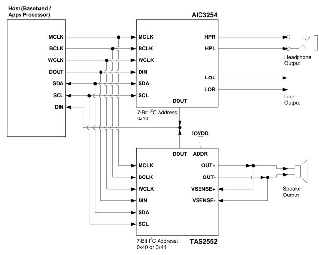
Figure 44. Configuration with TAS2552 and AIC3254 Muxed in TDM Mode
