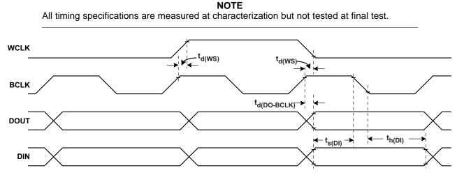
Figure 41. DSP Timing in Master Mode
