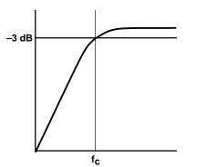
$f_{c(highpass)} = \frac{1}{2\pi R_{I}C_{I}}$  (8)
