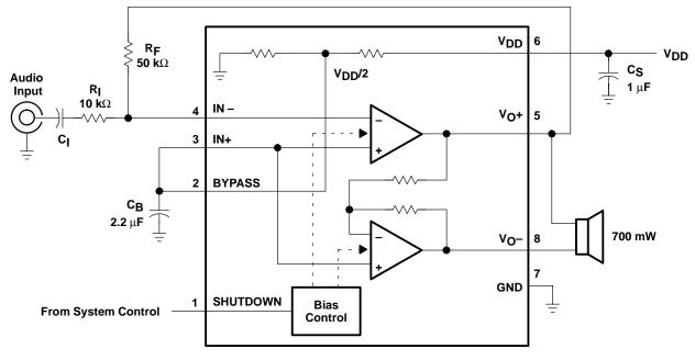
Figure 26. TPA701 Application Circuit
