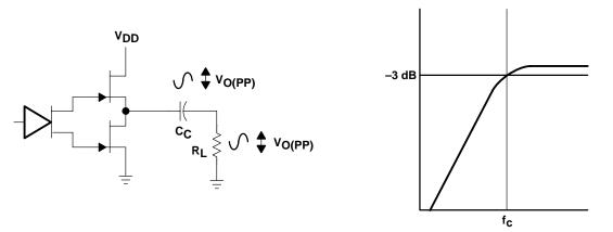
Figure 24. Single-Ended Configuration and Frequency Response
