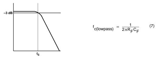
For example, if  $R_F$  is 100 k $\Omega$  and  $C_F$  is 5 pF, then  $f_{co}$  is 318 kHz, which is well outside of audio range.
