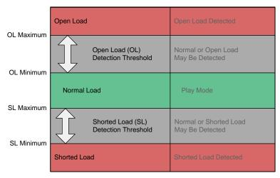
Figure 20. DC Load Diagnostic Reporting Thresholds
