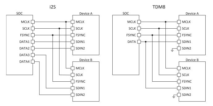
Figure 15. Digital-Audio Data Connection
