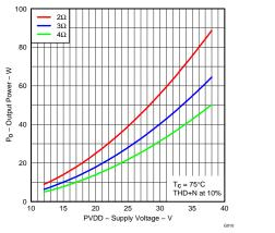
Figure 21. Output Power vs Supply Voltage
