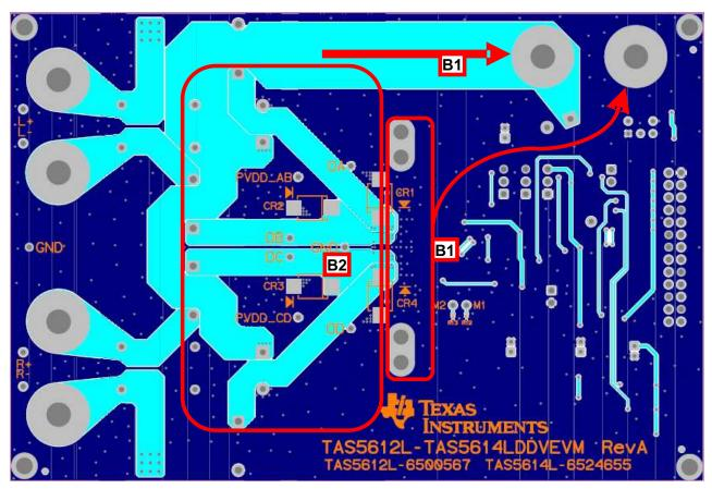
**Note B1**: A wide PVDD bus and a wide ground path must be used to provide very low impedance to high power and audio currents to the power supply. Top and bottom ground planes must be connected with vias at many points to reinforce the ground connections.
