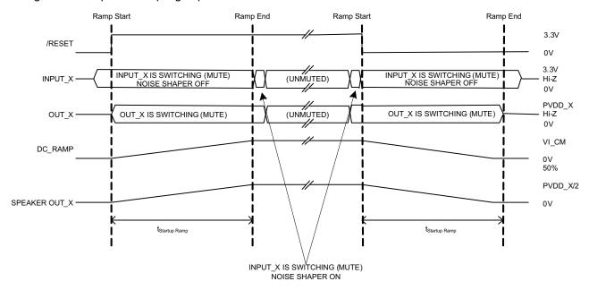
Figure 15. Start-up/Shutdown Ramp
