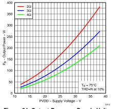
Figure 24. Output Power vs Supply Voltage
