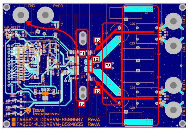
**Note T1**: Bottom and top layer ground plane areas are used to provide strong ground connections. The area under the IC must be treated as central ground, with IC grounds connected there and a strong via matrix connecting the area to bottom ground plane. The ground path from the IC to the power supply ground through top and bottom layers must be strong to provide very low impedance to high power and audio currents.
