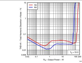
Figure 17. Total Harmonic + Noise vs Output Power, 1 kHz
