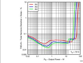
Figure 20. Total Harmonic Distortion + Noise vs Output Power
