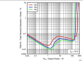
Figure 11. Total Harmonic Distortion + Noise vs Output Power
