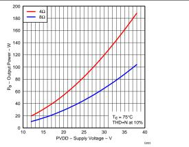
Figure 18. Output Power vs Supply Voltage vs Distortion + Noise = 10%
