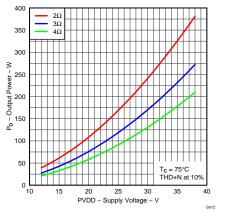
Figure 12. Output Power vs Supply Voltage
