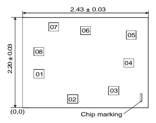
Chip making (X=2,283, Y=0,165) 20 Size pad: 0.12 x 0.12 mm
