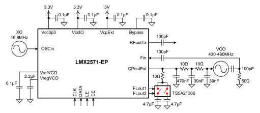
Figure 8-22. Typical PLL Duplex Mode Application Schematic
