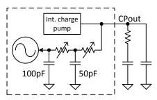
Figure 7-2. Integrated Loop Filter
