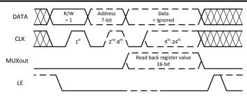
Figure 7-6. Register Readback Timing Diagram
