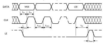
Figure 6-1. MICROWIRE Timing Diagram
