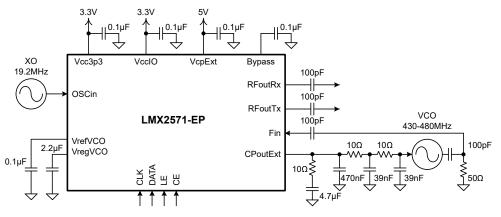
Figure 8-28. Typical Synthesizer/PLL Duplex Mode Application Schematic
