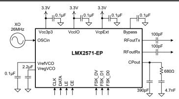
Figure 8-12. Typical Synthesizer Duplex Mode Application Schematic
