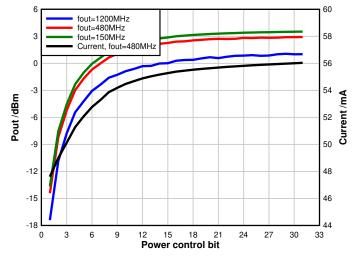
Figure 8-11. Configurable RF Output Power
