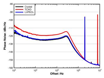
Figure 8-10. Phase Noise vs. Input Clock
