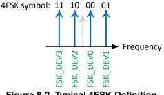
Figure 8-2. Typical 4FSK Definition
