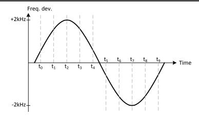
Figure 8-3. Over-Sampling Modulation Signal
