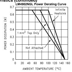
This curve shows the LM4902NGL's thermal dissipation ability at different ambient temperatures given the exposed-DAP of the part is soldered to a plane of 1oz. Cu with an area given in the label of each curve.
