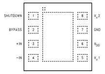
Figure 2. VSSOP - Top View See Package Number DGK
