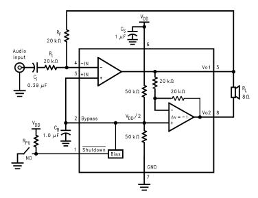
Figure 1. Typical Audio Amplifier Application Circuit
