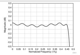
Figure 39. Linear Phase Decimation Filter Magnitude Response
