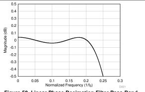
Figure 49. Linear Phase Decimation Filter Magnitude Response
