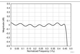
Figure 46. Linear Phase Decimation Filter Pass-Band Ripple
