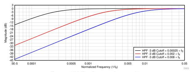
Figure 33. HPF Filter Frequency Response Plot
