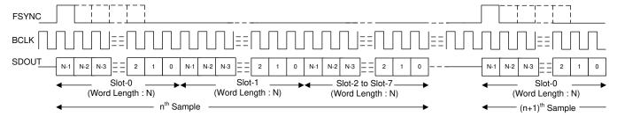
Figure 17. TDM Mode Standard Protocol Timing (TX OFFSET = 0)
