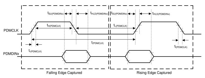
Figure 4. PDM Digital Microphone Interface Timing Diagram
