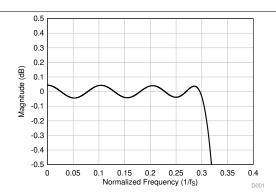
Figure 48. Linear Phase Decimation Filter Pass-Band
