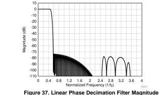
Figure 37. Linear Phase Decimation Filter Magnitude Response
