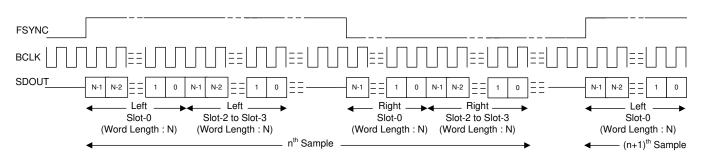
Figure 25. LJ Mode Standard Protocol Timing (TX\_OFFSET = 0)
