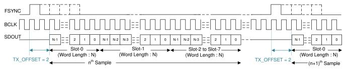
Figure 18. TDM Mode Protocol Timing (TX\_OFFSET = 2)
