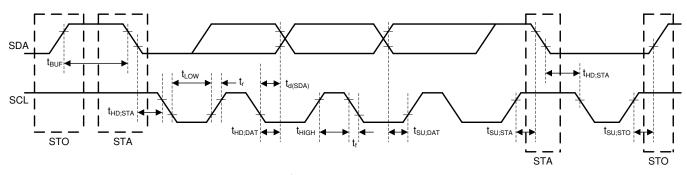
Figure 1. I<sup>2</sup>C Interface Timing Diagram
