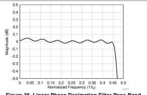
Figure 36. Linear Phase Decimation Filter Pass-Band Ripple
