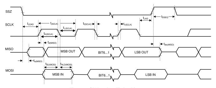
Figure 2. SPI Interface Timing Diagram
