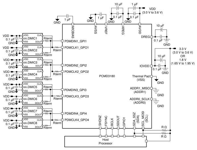
Figure 161. Eight-Channel Digital PDM Microphone Recording Diagram
