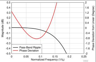
Figure 78. Ultra-Low-Latency Decimation Filter Pass-Band **Ripple and Phase Deviation**
