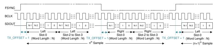
Figure 28. LJ Protocol Timing (TX\_OFFSET = 1 and BCLK\_POL = 1)
