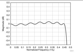
Figure 38. Linear Phase Decimation Filter Pass-Band Ripple
