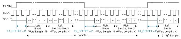
Figure 26. LJ Protocol Timing (TX\_OFFSET = 2)
