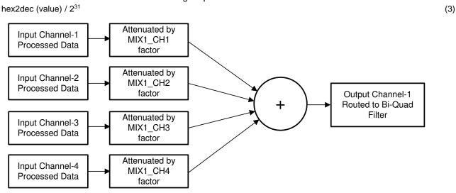
Figure 34. Programmable Digital Mixer Block Diagram
