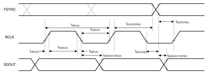
Figure 3. TDM (With BCLK\_POL = 1), I<sup>2</sup>S, and LJ Interface Timing Diagram
