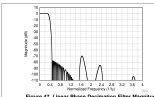
Figure 47. Linear Phase Decimation Filter Magnitude Response
