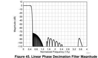
Figure 45. Linear Phase Decimation Filter Magnitude Response
