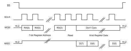
Figure 85. SPI Single-Byte Read Transfer
