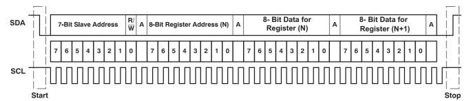
Figure 79. Typical I<sup>2</sup>C Sequence
