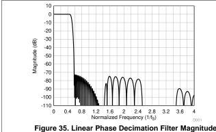
Figure 35. Linear Phase Decimation Filter Magnitude Response
