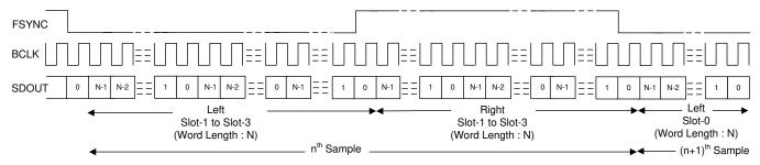
Figure 23. I2S Protocol Timing (No Idle BCLK Cycles, TX\_OFFSET = 0)
