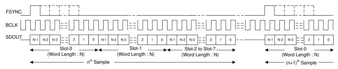
Figure 20. TDM Mode Protocol Timing (TX\_OFFSET = 0 and BCLK\_POL = 1)
