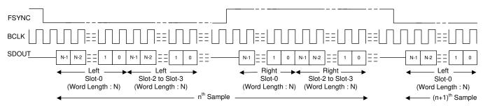
Figure 21. I<sup>2</sup>S Mode Standard Protocol Timing (TX\_OFFSET = 0)
