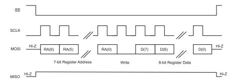
Figure 84. SPI Single-Byte Write Transfer
