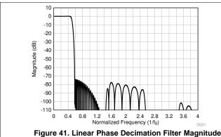
Figure 41. Linear Phase Decimation Filter Magnitude Response
