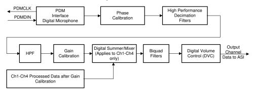
Figure 32. Signal-Chain Processing Flowchart
