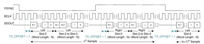
Figure 22. I<sup>2</sup>S Protocol Timing (TX\_OFFSET = 1)
