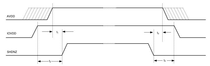
Figure 164. Power-Supply Sequencing Requirement Timing Diagram
