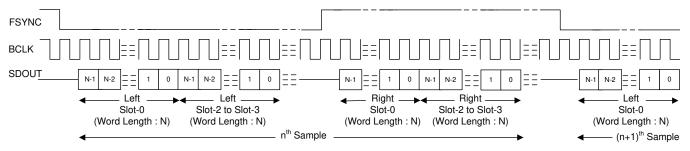
Figure 24. I<sup>2</sup>S Protocol Timing (TX\_OFFSET = 0 and BCLK\_POL = 1)
