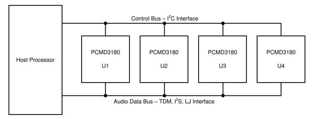
Figure 29. Multiple PCMD3180 Devices With Shared Control and Audio Data Buses
