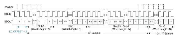
Figure 19. TDM Mode Protocol Timing (No Idle BCLK Cycles, TX OFFSET = 2)
