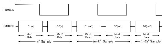
Figure 31. Digital PDM Microphone Protocol Timing Diagram
