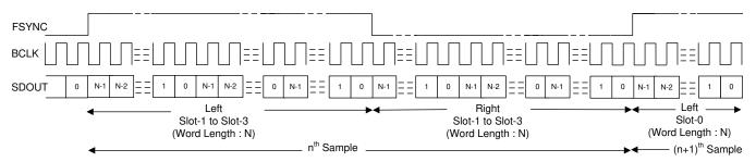
Figure 27. LJ Protocol Timing (No Idle BCLK Cycles, TX OFFSET = 0)
