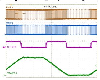
Figure 25. Signal Clipping PWM and Speaker Output Signals
