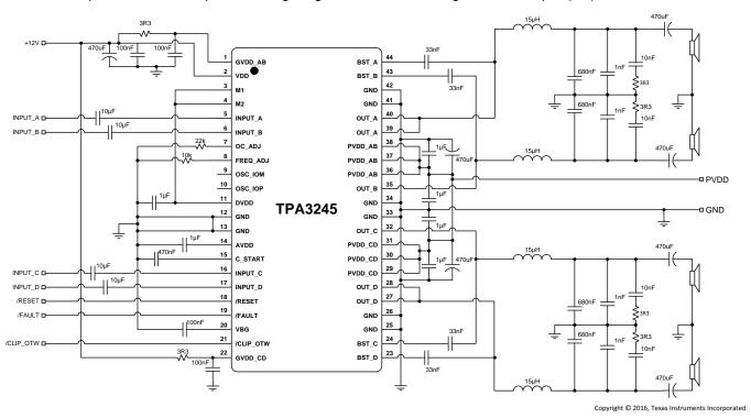
Figure 27. Typical Single Ended (1N) SE Application
