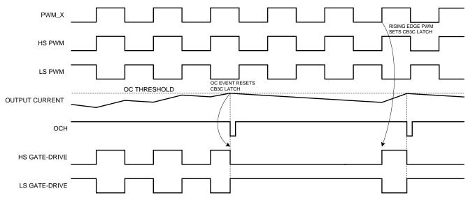
Figure 23. CB3C Timing Example
