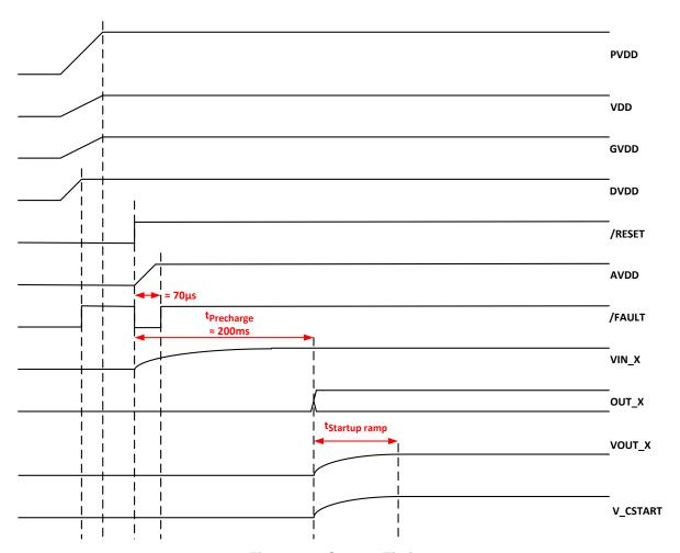
Figure 30. Startup Timing
