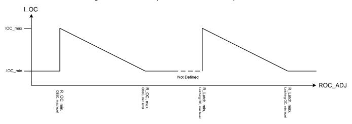
Figure 24. OC Threshold versus OC ADJ Resistor Value Example
