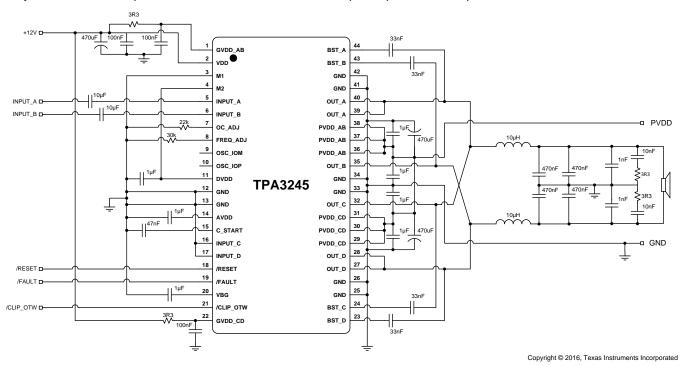
Figure 28. Typical Differential (2N) PBTL (Outputs Paralleled before LC filter) Application
