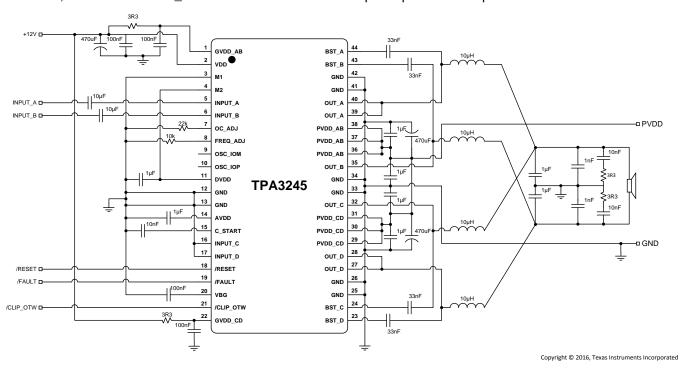
Figure 29. Typical Differential (2N) PBTL (Outputs Paralleled after LC filter) Application
