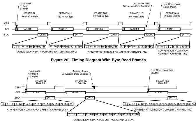
Figure 21. Timing Diagram With Word Read Frames
