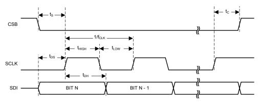
Figure 1. Serial Control Port Timing – Write
