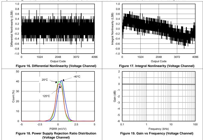
All plots at T<sub>A</sub> = 25°C, VDD = 5.0 V, VDIG = 5.0 V, VCM = 0 V and GND = DGND = 0 V, unless otherwise specified.
