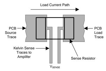
Figure 28. 4-Wire "Kelvin" Sensing Technique
