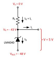
Figure 25. Shunt Regulator Voltages
