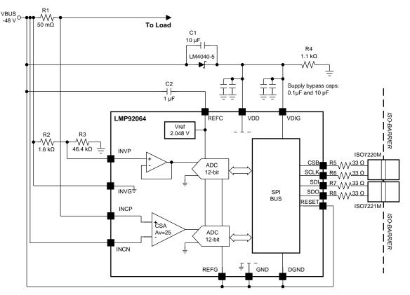
Figure 23. Typical Application Diagram
