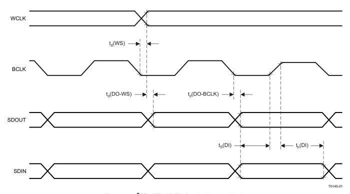
Figure 1. I<sup>2</sup>S/LJF/RJF Timing In Master Mode
