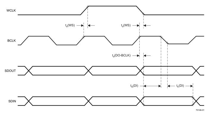
Figure 3. DSP Timing In Master Mode
