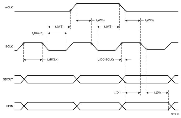
Figure 4. DSP Timing In Slave Mode
