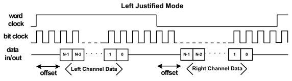
Figure 37. DSP Mode And Left Justified Modes, Showing The Effect Of A Programmed Data Word Offset
