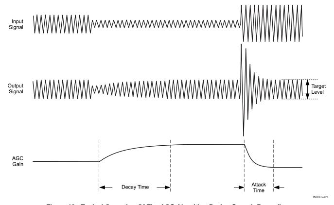
Figure 13. Typical Operation Of The AGC Algorithm During Speech Recording
