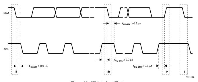
Figure 28. I<sup>2</sup>C Interface Timing
