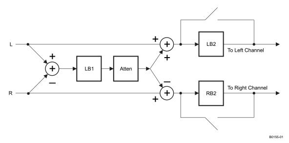
Figure 15. Architecture Of The Digital Audio Processing When 3D Effects Are Enabled
