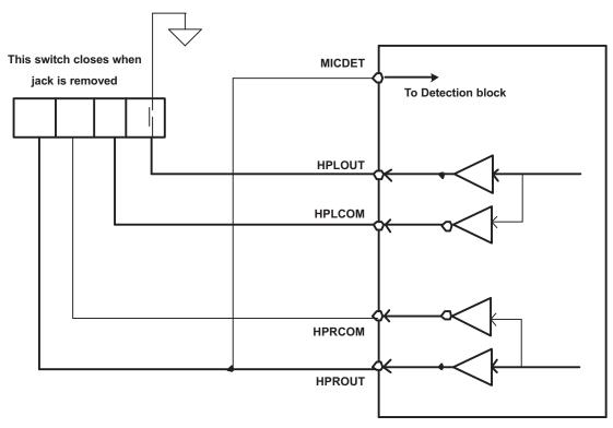
Figure 23. Configuration Of Device For Jack Detection Using A Fully Differential Stereo Headphone Output Connection
