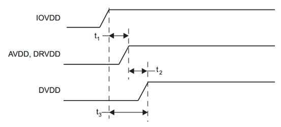
Figure 43. TLV320AIC3101 Power Supply Sequencing
