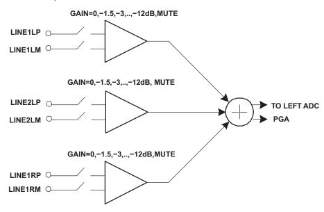
Figure 16. Left Channel Fully-Differential Analog Input Mixing Configuration
