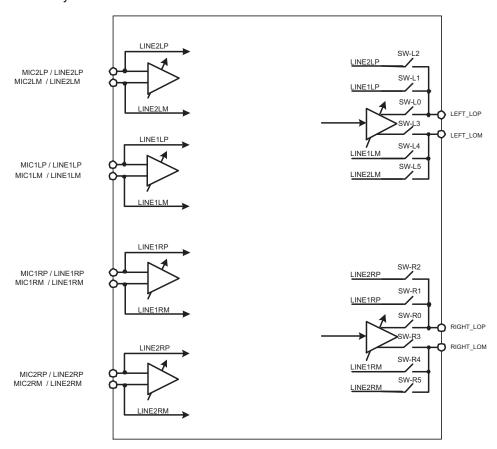
Figure 25. Passive Analog Bypass Mode Configuration
