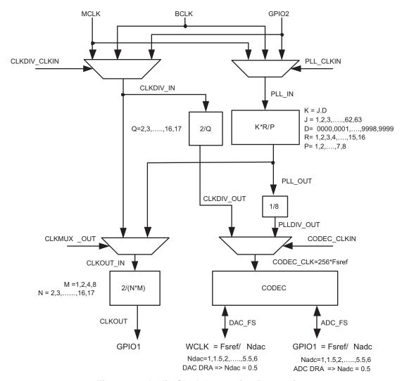
Figure 38. Audio Clock Generation Processing
