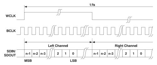
Figure 34. Left-Justified Serial Data Bus Mode Operation
