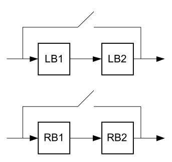
Figure 14. Structure Of The Digital Effects Processing For Independent Channel Processing
