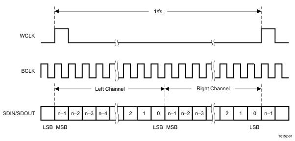
Figure 36. DSP Serial Bus Mode Operation
