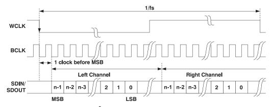
Figure 35. I<sup>2</sup>S Serial Data Bus Mode Operation
