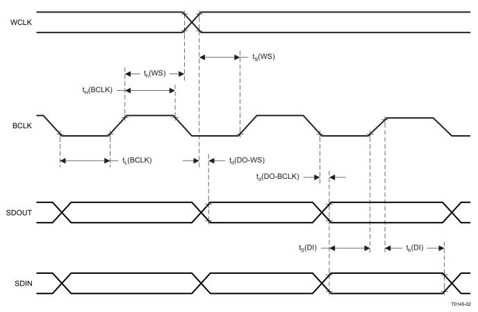
Figure 2. I<sup>2</sup>S/LJF/RJF Timing In Slave Mode
