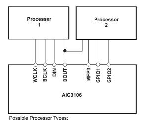
Application Processor, Multimedia Processor, Compressed Audio Decoder, Wireless Modem, Bluetooth Module, Additional Audio/Voice Codec
