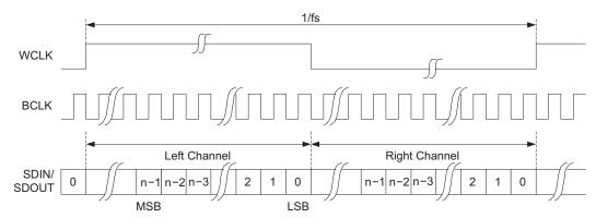
Figure 33. Right-Justified Serial Bus Mode Operation
