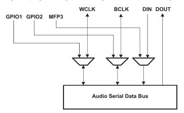
Figure 31. Alternate Audio Bus Mulitplexing Function
