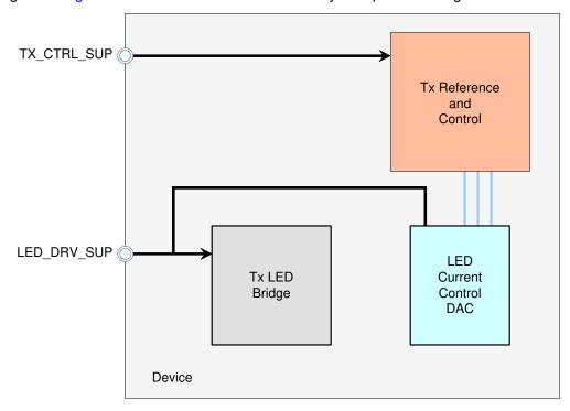
Figure 8-19. Transmit Subsystem Power Routing
