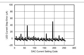
Figure 7-30. Transmitter DAC Current Step Error
