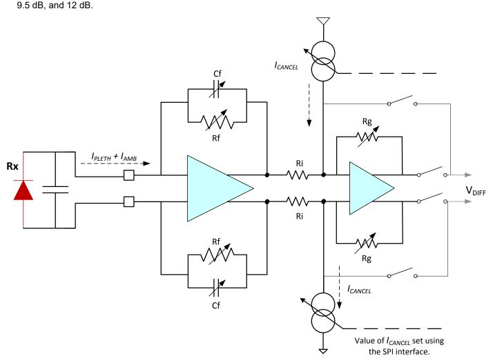
Figure 8-5. Front-End (I-V Amplifier and Cancellation Stage)
