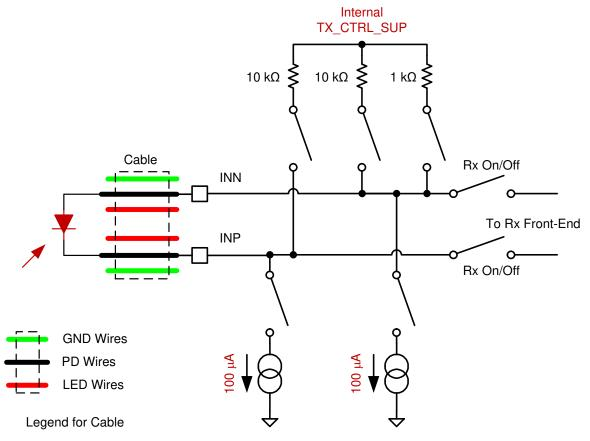
Figure 8-31. Photodiode Diagnostic
