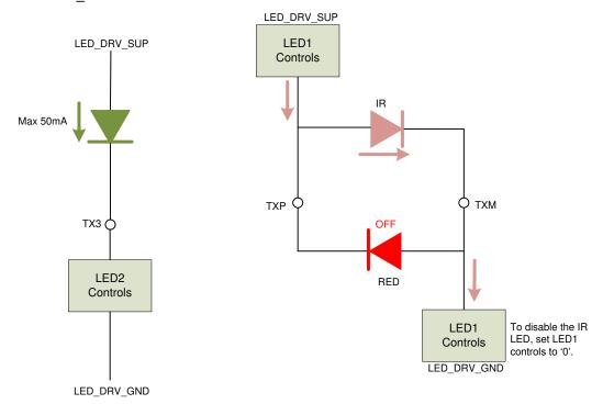
Figure 8-24. HRM Application Using the Third LED
