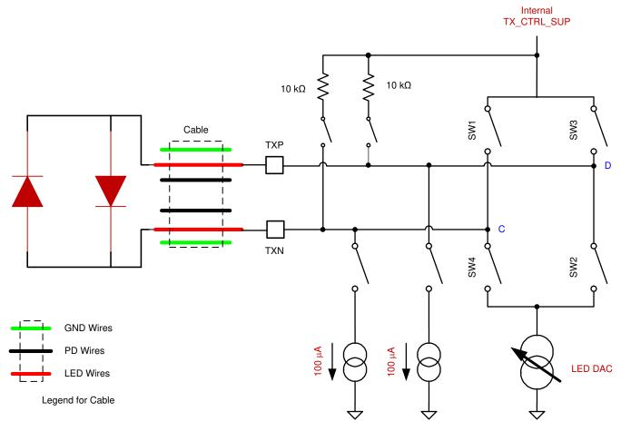
Figure 8-32. Transmitter Diagnostic
