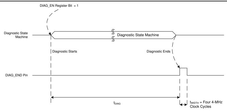
Figure 8-33. Diagnostic Timing Diagram
