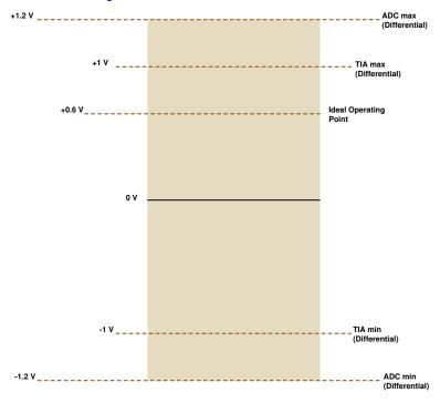
Figure 8-3. Signal Levels in TIA and ADC
