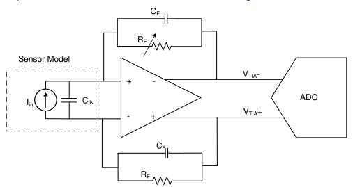
Figure 8-2. TIA Block Diagram
