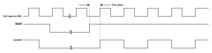
Figure 8-8. Clock Divider Reset
