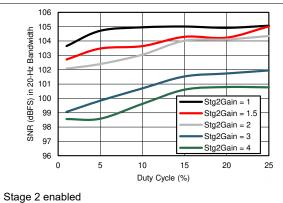
Figure 7-27. Receiver SNR over Nyquist Bandwidth vs Duty Cycle (Different Stage 2 Gain Settings)
