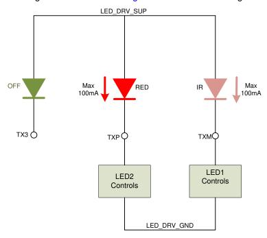
Figure 8-21. SPO2 Application, Common Anode Configuration
