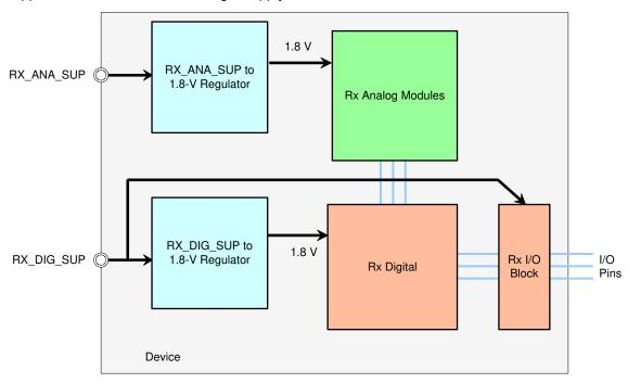
Figure 8-15. Receive Subsystem Power Routing
