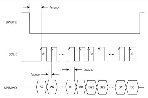
Figure 7-2. Serial Interface Timing Diagram, Write Operation
