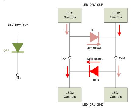
Figure 8-23. SPO2 Application, H-Bridge Configuration
