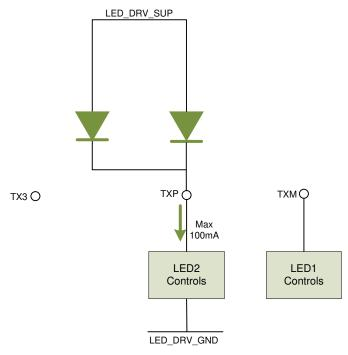
Figure 8-25. Using Two Parallel LEDs for an HRM Application
