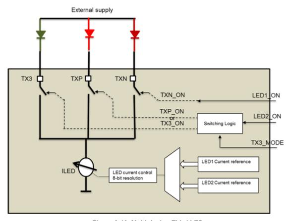
Figure 8-18. Multiplexing Third LED
