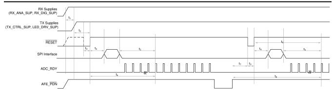
Figure 7-3. Supply Ramp and Hardware Power-Down Timing
