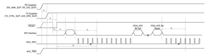
Figure 7-4. Supply Ramp and Software Power-Down Timing
