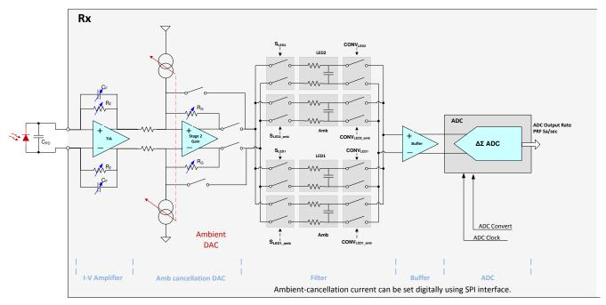
Figure 8-1. Receiver Front-End
