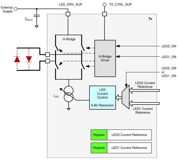
Figure 8-16. Transmit: H-Bridge Drive
