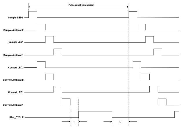
Figure 8-30. Dynamic Power-Down Mode Timing
