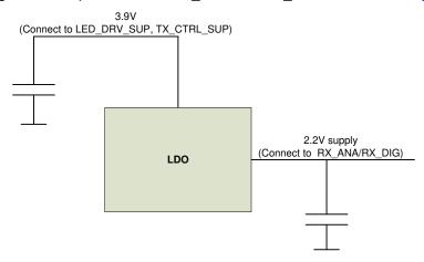
Figure 10-2. Buck Converter or an LDO
