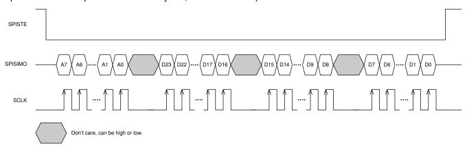
Figure 8-34. AFE SPI Write Timing Diagram
