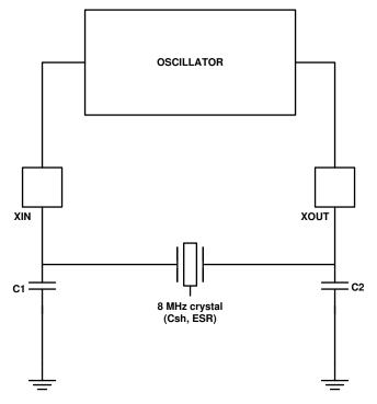
Figure 8-9. Connection of Crystal to AFE4403
