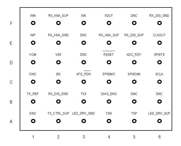
Figure 6-1. YZP Package, DSBGA-36, (Bottom View)
