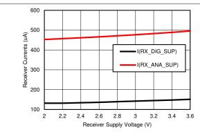
Figure 7-5. Receiver Currents vs Receiver Supply Voltage
