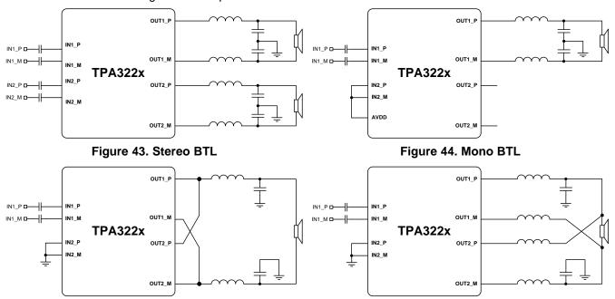
Figure 45. Mono PBTL, Pre LC Filter
