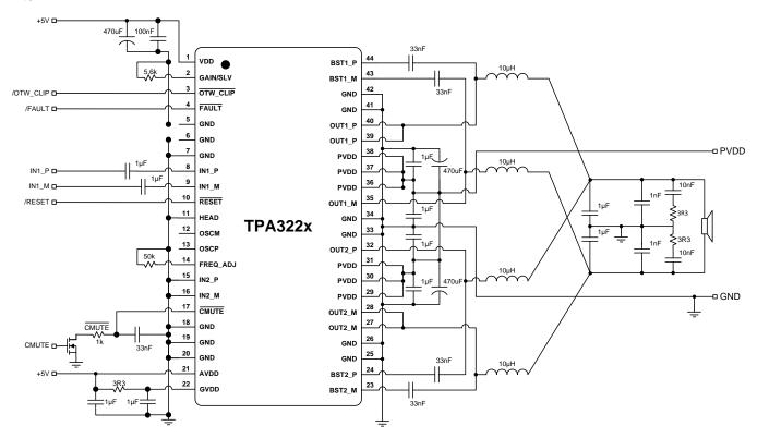
Figure 52. Typical Differential (2N) AD-Mode PBTL Application
