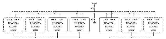
Figure 33. Gain and Master PCB Implementation
