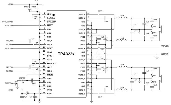
Figure 50. Typical Differential (2N) AD-Mode BTL Application
