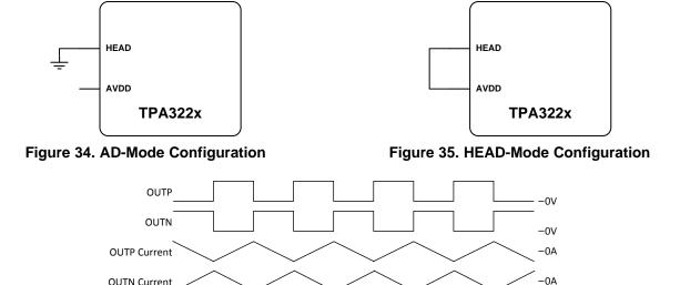
Figure 36. AD Mode Output Waveforms, Idle
