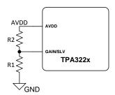
Figure 32. Gain and Master / Slave Setup
