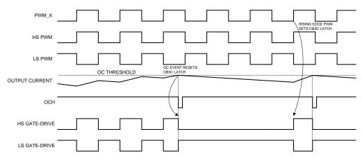
Figure 48. CB3C Timing Example
