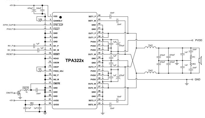
Figure 51. Typical Differential (2N) AD-Mode PBTL Application
