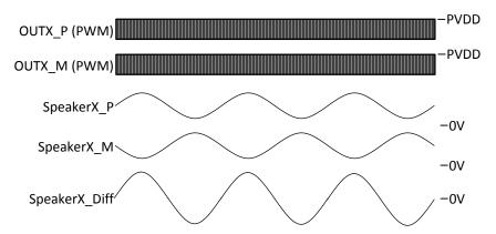
Figure 41. HEAD Mode Speaker Output Signals, Low Level Output
