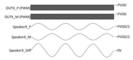
Figure 38. AD Mode Speaker Output Signals, Low or and High Level Output
