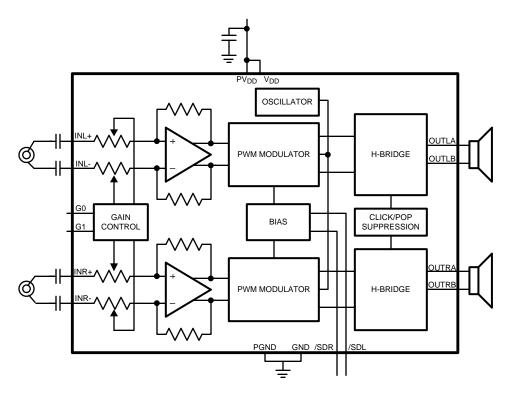
Figure 24. Differential Input Configuration
