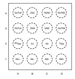
Figure 2. DSBGA - Top View See YZR0016 Package
