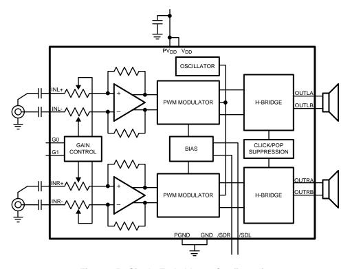
Figure 25. Single-Ended Input Configuration
