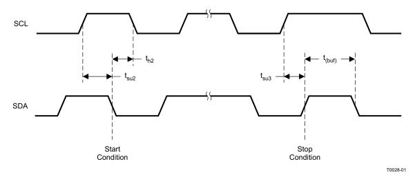
Figure 2. Timing for Start and Stop Conditions
