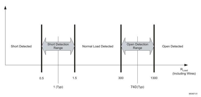
Figure 11. Open- and Shorted-Load Detection
