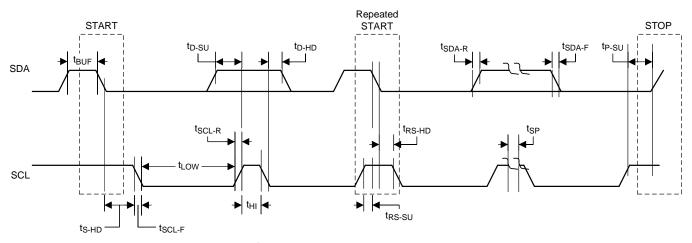
Figure 21. I<sup>2</sup>C Communication Port Timing Diagram
