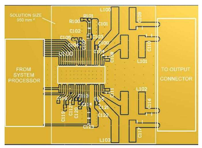
Figure 89. 2.0 (Stereo BTL) Top Copper View
