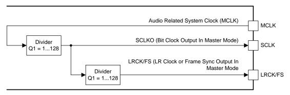
Figure 58. Simplified Clock Tree for MCLK Sourced Master Mode
