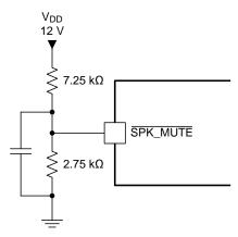
Figure 66. SPK\_MUTE Used in External Undervoltage Error Protection
