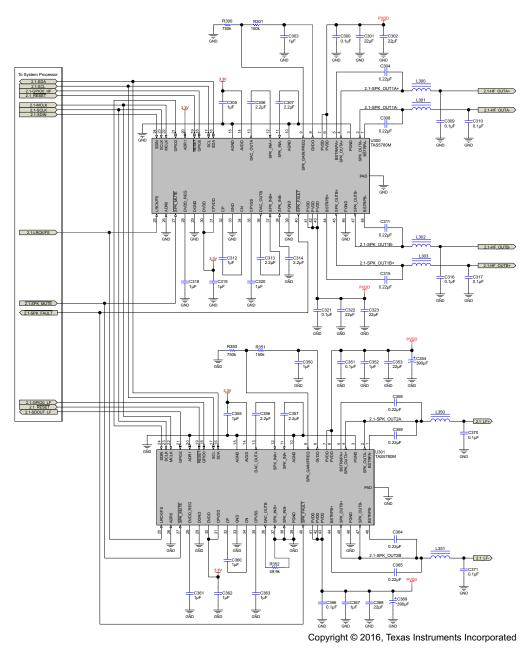
Figure 86. 2.1 (Stereo BTL + External Mono Amplifier) Application Schematic
