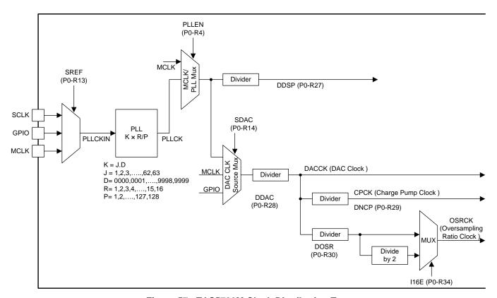
Figure 57. TAS5780M Clock Distribution Tree
