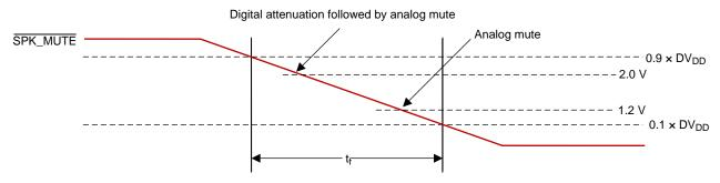
Figure 67. SPK\_MUTE Timing for External Undervoltage Error Protection
