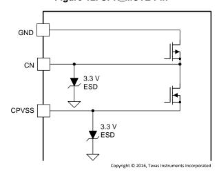
Figure 14. CN and CPVSS Pins
