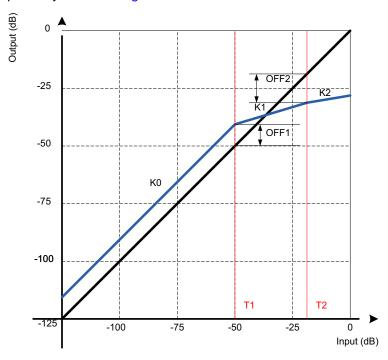
Figure 79. DRC Transfer Function Example Plot
