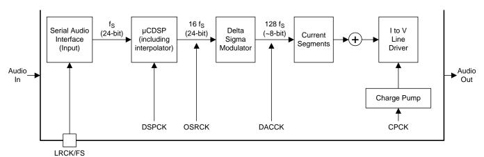
Figure 56. Audio Flow with Respective Clocks
