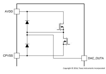
Figure 8. DAC\_OUTx Pins
