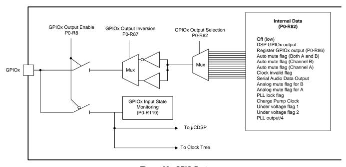
Figure 68. GPIO Port
