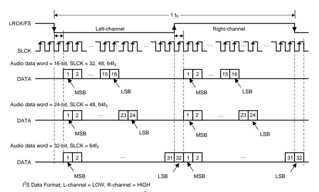
Figure 61. I<sup>2</sup>S Audio Data Format
