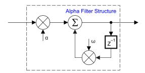
Figure 82. AGL Alpha Filter Structure
