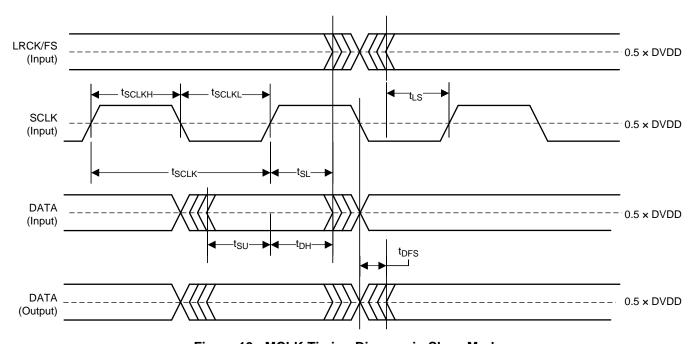
Figure 19. MCLK Timing Diagram in Slave Mode
