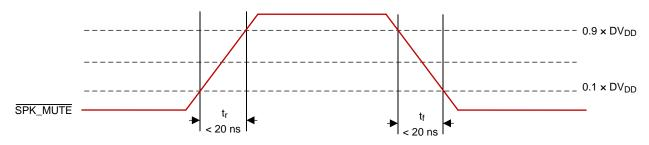
Figure 22. SPK\_MUTE Timing Diagram for Soft Mute Operation via Hardware Pin
