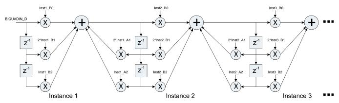
Figure 74. Cascaded BQ Structure
