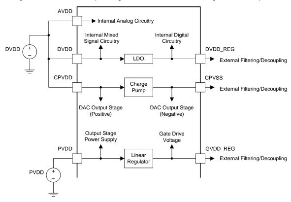
Figure 87. Power Supply Functional Block Diagram
