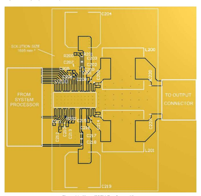
Figure 91. Mono (PBTL) Top Copper View
