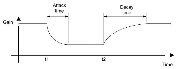
Figure 80. DRC Attack and Decay
