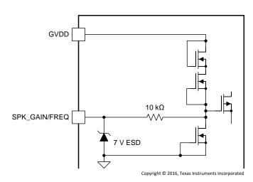
Figure 6. SPK\_GAIN/FREQ Pin
