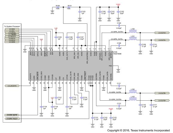
Figure 84. 2.0 (Stereo BTL) System Application Schematic
