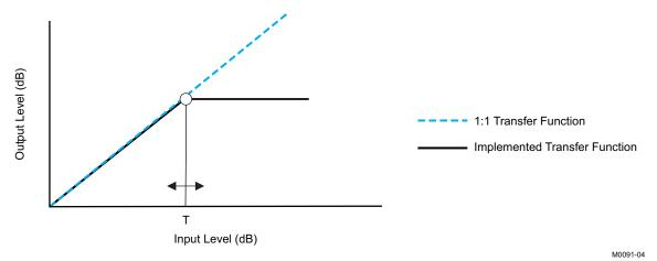
Figure 81. AGL Transfer Function Example Plot
