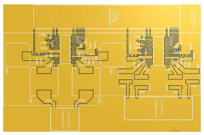
Figure 93. 2.1 (Stereo BTL + Mono PBTL) Top Copper View
