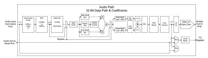
Figure 72. Fixed-Function Process Flow found in the TAS5780M
