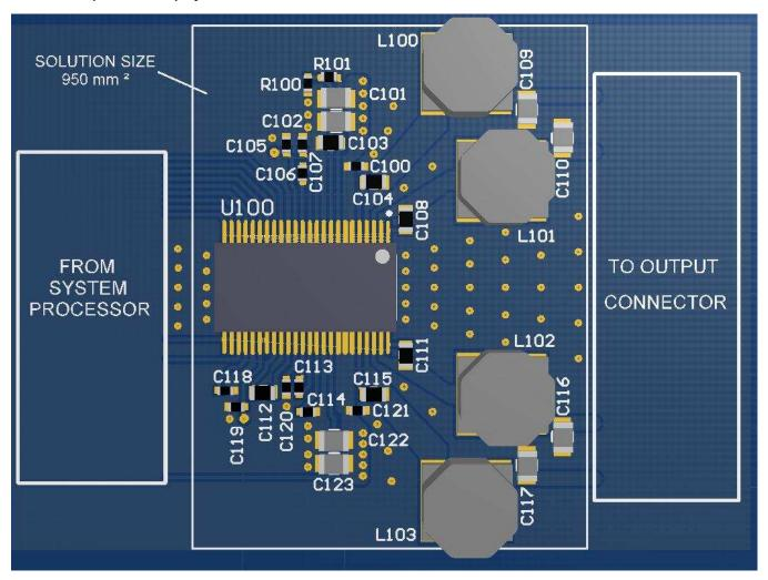
Figure 88. 2.0 (Stereo BTL) 3-D View
