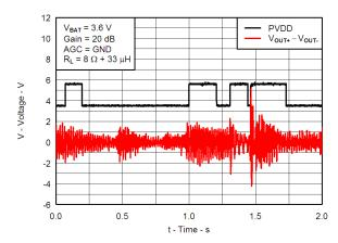
Figure 23. Adaptive Boost Converter with Typical Music Playback
