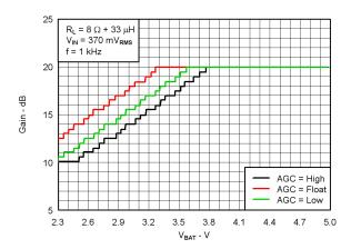
Figure 22. Gain vs Battery voltage
