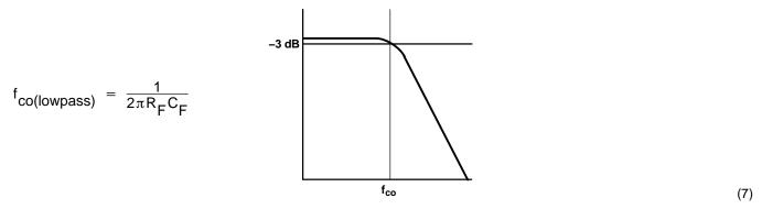
For example, if  $R_F$  is 100 k $\Omega$  and  $C_F$  is 5 pF then  $f_{co}$  is 318 kHz, which is well outside the audio range.
