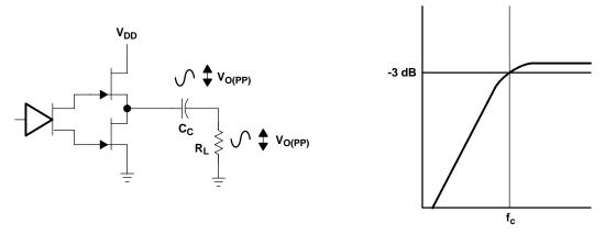
Figure 24. Single-Ended Configuration and Frequency Response
