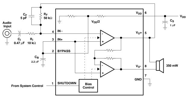
Figure 26. TPA301 Application Circuit
