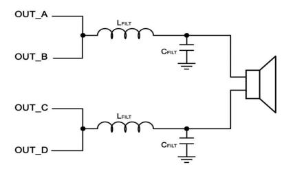
Figure 58. Post-Filter PBTL
