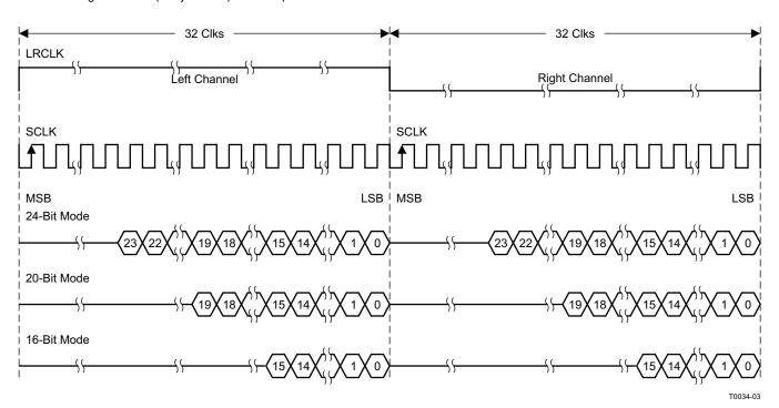
Figure 52. Right-Justified 64-F<sub>S</sub> Format
