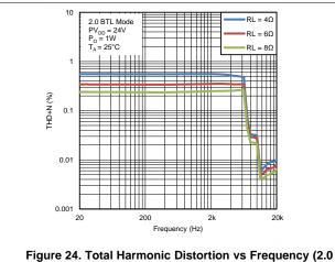
Figure 24. Total Harmonic Distortion vs Frequency (2.0 BTL Mode)
