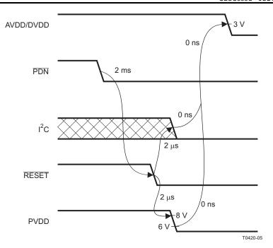
Figure 70. Power-Loss Sequence
