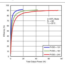
Figure 25. Efficiency vs Output Power (2.0 BTL Mode)
