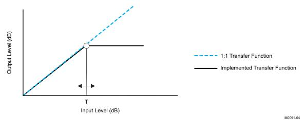
Professional-quality dynamic range compression automatically adjusts volume to flatten volume level.
