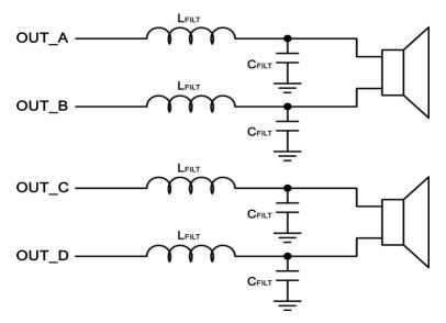
Figure 57. Stereo BTL Mode
