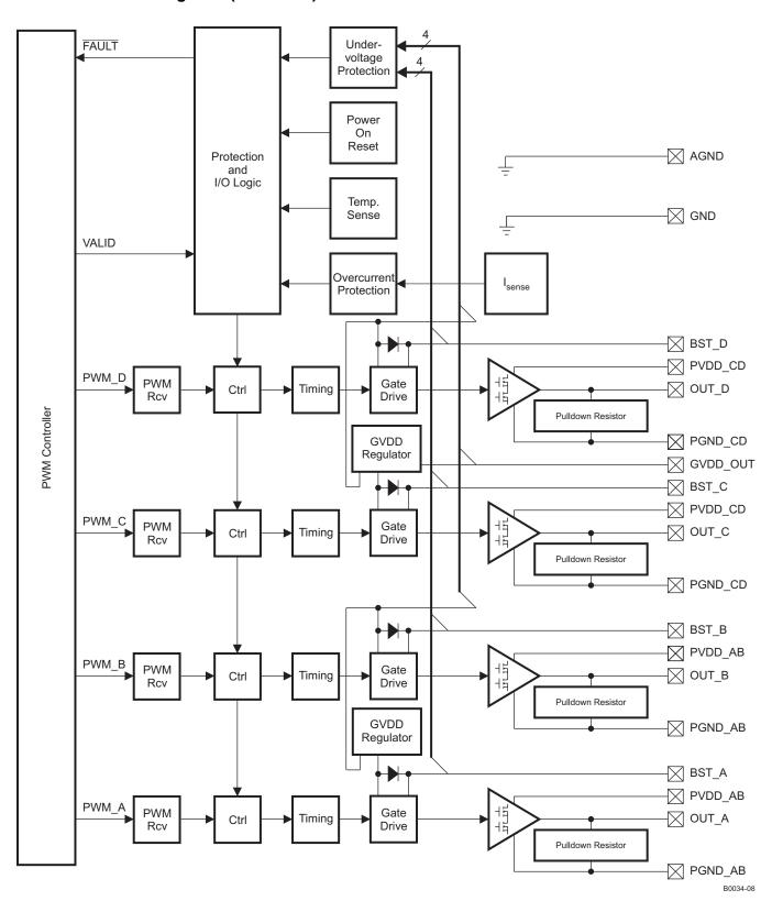
Figure 44. Power-Stage Functional Block Diagram
