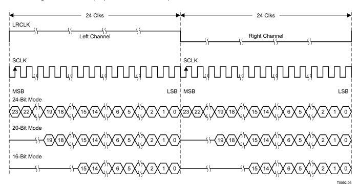
Figure 53. Right-Justified 48-F<sub>S</sub> Format
