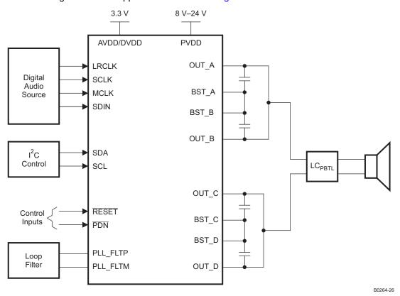
Figure 71. Mono Parallel Bridge Tied Load Application
