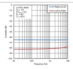
Figure 26. Crosstalk vs Frequency (2.0 BTL Mode)
