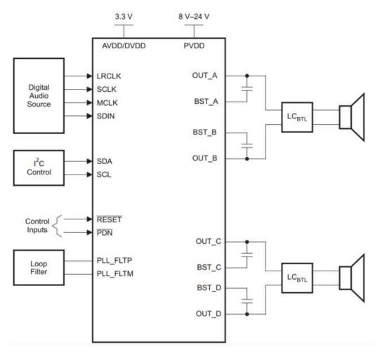
Figure 68. Stereo Bridge Tied Load Application
