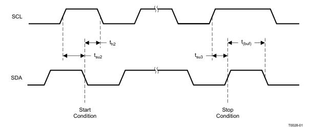
Figure 3. Start and Stop Conditions Timing
