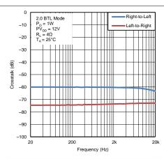
Figure 28. Crosstalk vs Frequency (2.0 BTL Mode)
