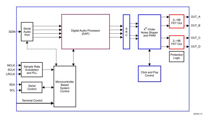
Figure 43. Functional Block Diagram
