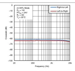
Figure 29. Crosstalk vs Frequency (2.0 BTL Mode)
