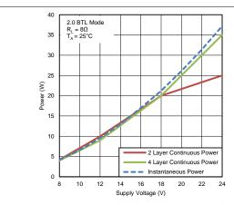
Figure 30. Power vs Supply Voltage (2.0 BTL Mode)
