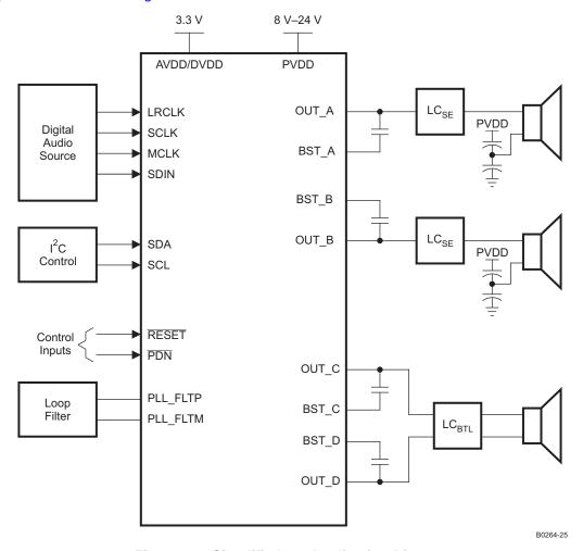
Figure 72. Simplified 2.1 Application Diagram
