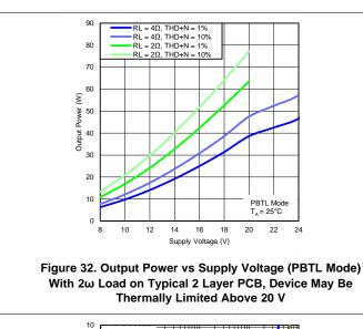
With 2ω Load on Typical 2 Layer PCB, Device May Be
