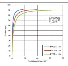
Figure 13. Efficiency vs Total Output Power (2.1 SE Mode)
