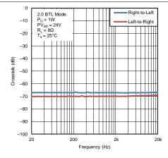
Figure 27. Crosstalk vs Frequency (2.0 BTL Mode)
