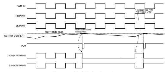
Figure 22. CB3C Timing Example
