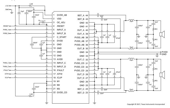
Figure 26. Typical Differential (2N) BTL Application
