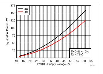
Figure 34. Output Power vs Supply Voltage
