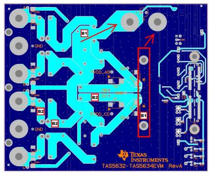
**Note B1**: A wide PVDD bus and a wide ground path must be used to provide very low impedance to high power and audio currents to the power supply. Top and bottom ground planes must be connected with vias at many points to reinforce the ground connections.
