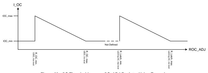
Figure 23. OC Threshold versus OC\_ADJ Resistor Value Example
