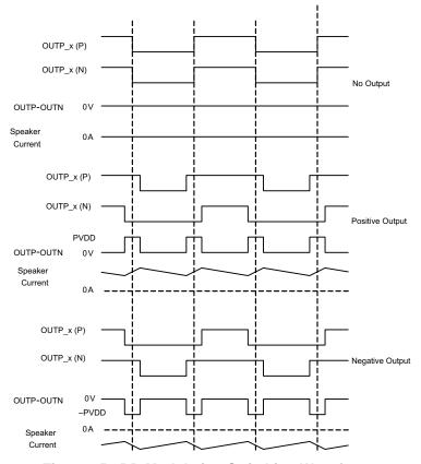
Figure 25. BD Modulation Switching Waveforms
