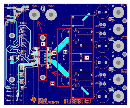
**Note T1**: Bottom and top layer ground plane areas are used to provide strong ground connections. The area under the IC must be treated as central ground, with IC grounds connected there and a strong via matrix connecting the area to bottom ground plane. The ground path from the IC to the power supply ground through top and bottom layers must be strong to provide very low impedance to high power and audio currents.
