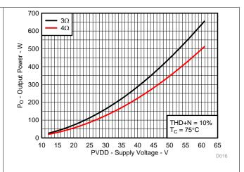
Figure 31. Output Power vs Supply Voltage
