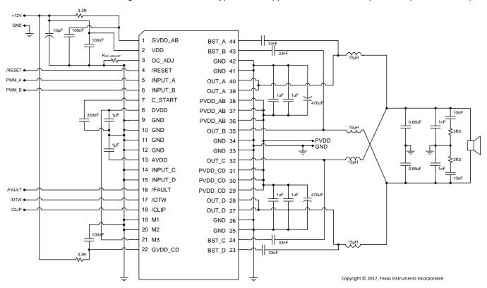
Figure 29. Typical Differential (2N) PBTL Application
