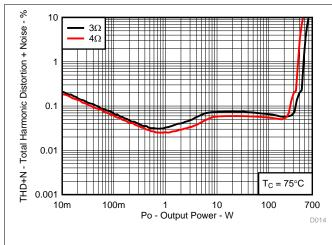
Figure 30. Total Harmonic Distortion + Noise vs Output Power
