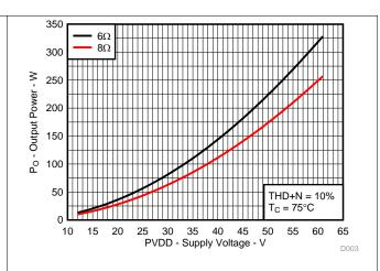
Figure 28. Output Power vs Supply Voltage
