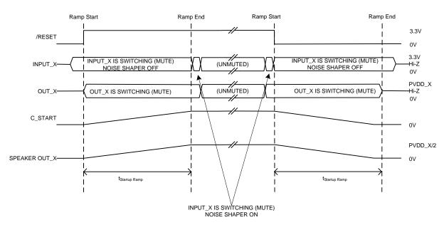
Figure 21. Start-Up and Shutdown Ramp
