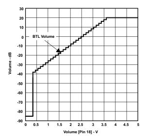
Figure 24. Typical DC Volume Control Operation
