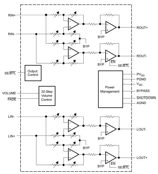
NOTE: All resistor wipers are adjusted with 32 step volume control.
