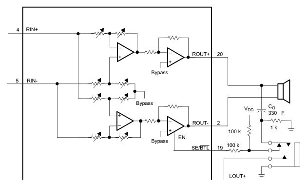
Figure 21. TPA6021A4 Resistor Divider Network Circuit
