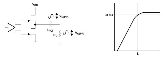
Figure 27. Single-Ended Configuration and Frequency Response
