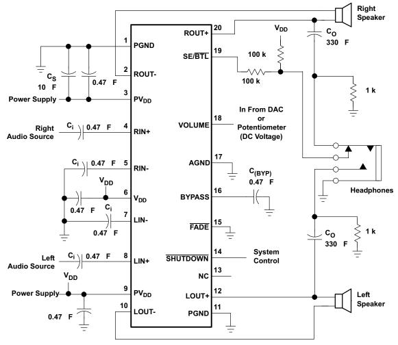
A. A 0.47-µF ceramic capacitor should be placed as close as possible to the IC. For filtering lower-frequency noise signals, a larger electrolytic capacitor of 10 µF or greater should be placed near the audio power amplifier.
