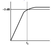
The value of  $C_l$  is important to consider as it directly affects the bass (low frequency) performance of the circuit. Consider the example where  $R_l$  is 70 k $\Omega$  and the specification calls for a flat-bass response down to 40 Hz. Equation 2 is reconfigured as Equation 3.
