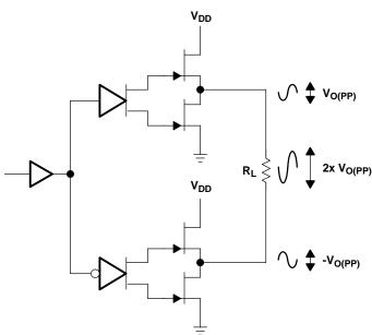
Figure 26. Bridge-Tied Load Configuration
