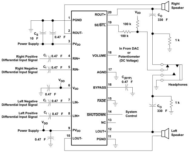
A. A 0.47-µF ceramic capacitor should be placed as close as possible to the IC. For filtering lower-frequency noise signals, a larger electrolytic capacitor of 10 µF or greater should be placed near the audio power amplifier.
