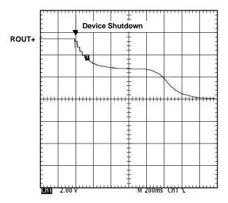
Figure 22. Shutdown Sequence in the Fade-on Mode
