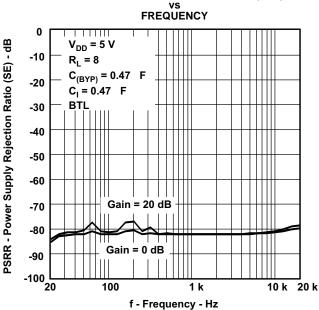
POWER SUPPLY REJECTION RATIO (BTL)
