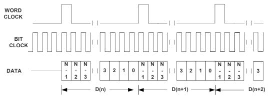
Figure 39. Timing Diagram for Mono PCM Mode
