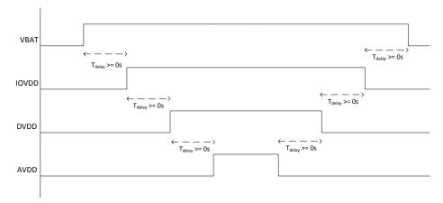
Figure 150. Power Supply Sequence for Power-Up and Power-Down
