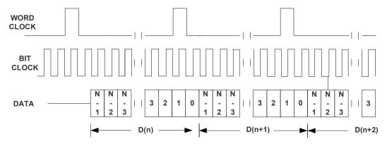
Figure 41. Timing Diagram for Mono PCM Mode with ASI\_OFFSET1=2 and Bit Clock Inverted
