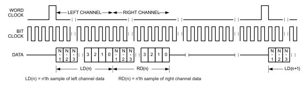
Figure 33. Timing Diagram for DSP Mode with ASI\_OFFSET1=1
