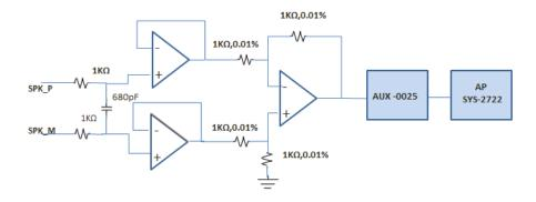
Figure 18. Differential To Single-Ended (D2S) Filter
