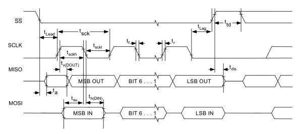
Figure 2. SPI Interface Timing Diagram
