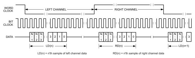
Figure 31. Timing Diagram for I<sup>2</sup>S Mode with ASI\_OFFSET1 = 0 and Inverted Bit Clock
