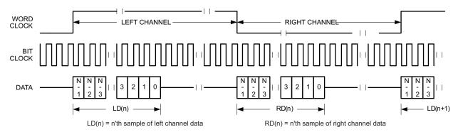
Figure 36. Timing Diagram for Left-Justified Mode
