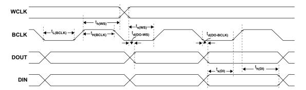
Figure 4. I<sup>2</sup>S/LJF/RJF Timing in Slave Mode
