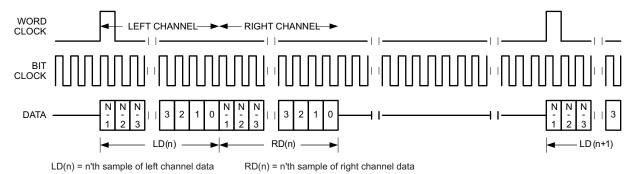
Figure 32. Timing Diagram for DSP Mode
