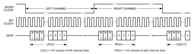
Figure 29. Timing Diagram for I<sup>2</sup>S Mode
