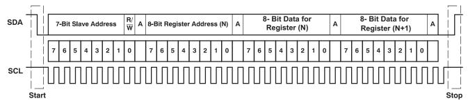
Figure 19. Typical I<sup>2</sup>C Sequence
