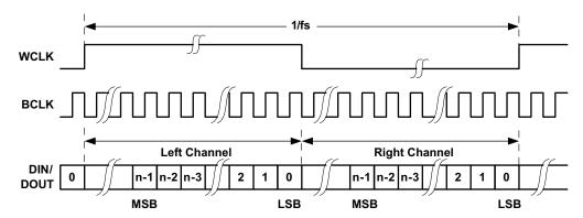
Figure 35. Timing Diagram for Right-Justified Mode
