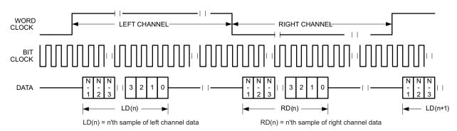
Figure 37. Timing Diagram for Light-Left Mode with ASI\_OFFSET1 = 1
