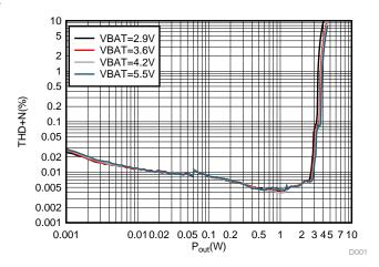
Freq = 1kHz VBAT = 3.6 V, AVDD = IOVDD = 1.8 V,  $\overline{RESET}$  = IOVDD,  $R_L$  = 8  $\Omega$  + 33  $\mu$ H, I2S digital input, ROM mode 1
