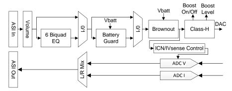
Figure 28. ROM Mode 2 Processing Block Diagram
