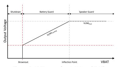
Figure 25. VLIM versus Supply Voltage (VBAT)
