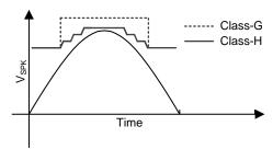
Figure 26. Boost Mode Signal Tracking Example
