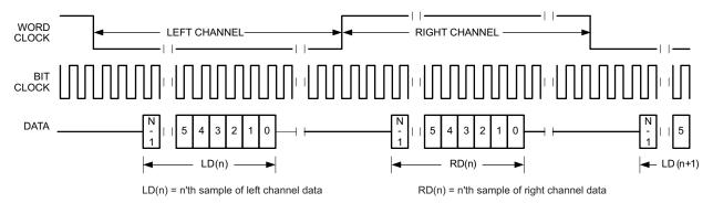
Figure 42. Timing Diagram for I<sup>2</sup>S in TDM Mode with ASI OFFSET1=2
