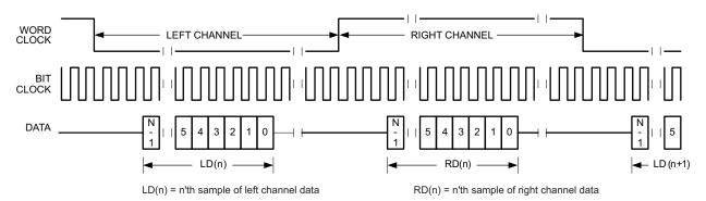
Figure 30. Timing Diagram for I2S Mode with ASI OFFSET1 = 2
