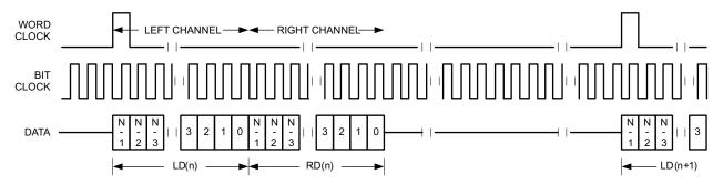
Figure 34. Timing Diagram for DSP Mode with ASI OFFSET1=0 and Inverted Bit Clock
