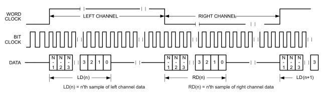
Figure 38. Timing Diagram for Left-Justified Mode with ASI\_OFFSET1 = 0 and Inverted Bit Clock
