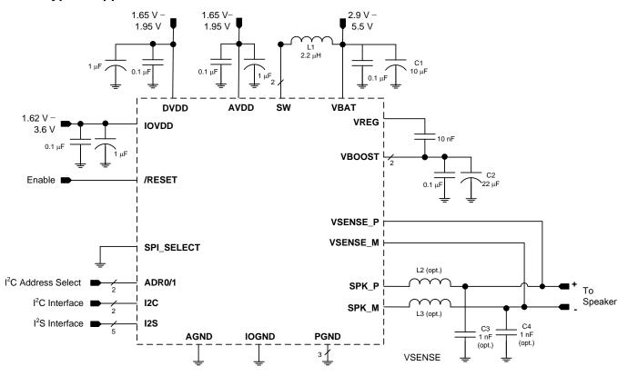
Figure 148. Typical Application - Digital Audio Input
