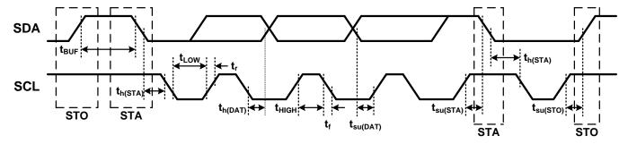
Figure 1. I<sup>2</sup>C Timing
