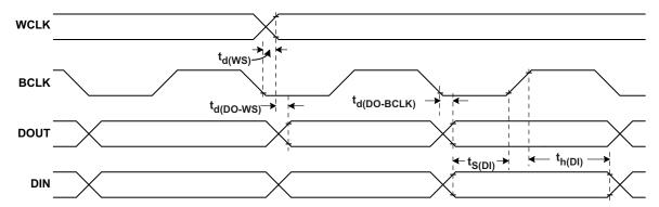
Figure 3. I<sup>2</sup>S/LJF/RJF Timing in Master Mode
