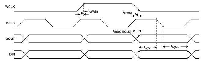
Figure 5. DSP Timing in Master Mode
