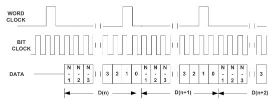
Figure 40. Timing Diagram for Mono PCM Mode with ASI\_OFFSET1=2
