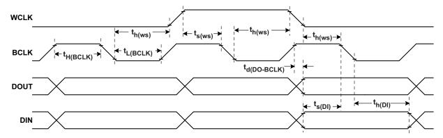
Figure 6. DSP Timing in Slave Mode
