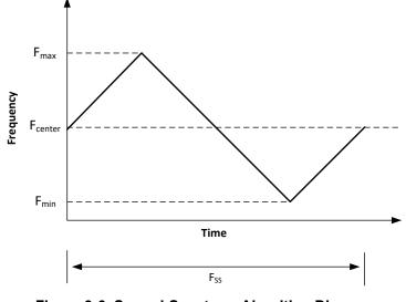
Figure 9-6. Spread-Spectrum Algorithm Diagram
