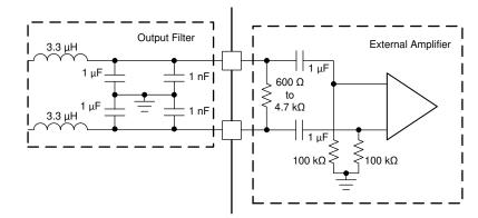
Figure 10-1. External Amplifier Input Configuration for Line Driver
