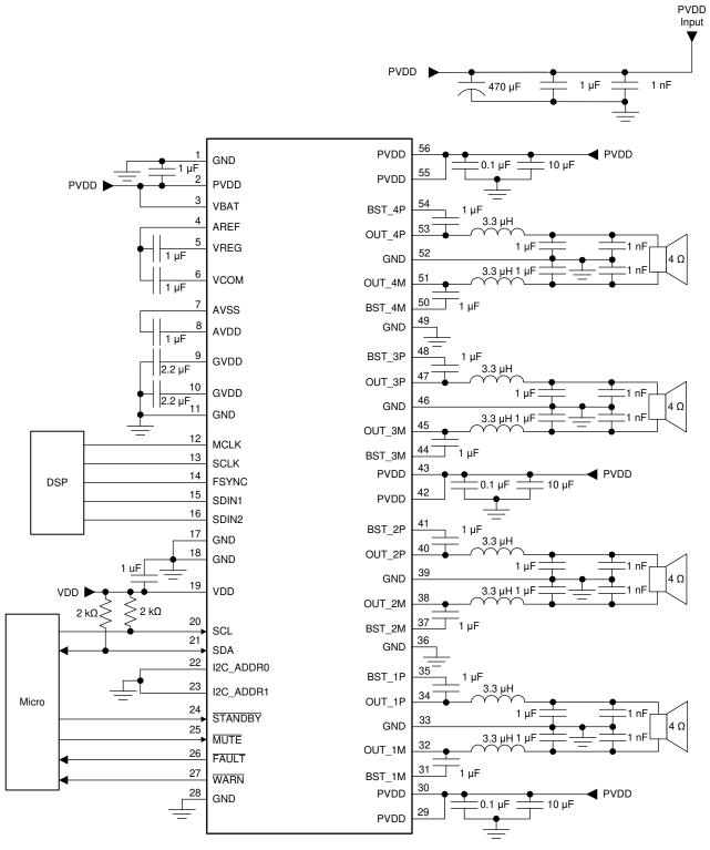
Figure 10-2. Typical 4-Channel BTL Application Schematic
