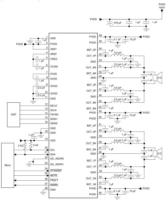
Figure 10-3. Typical 2-Channel PBTL Application Schematic
