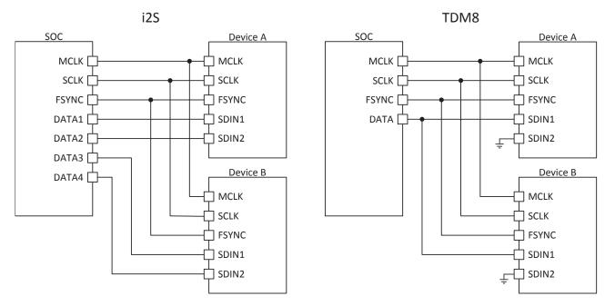
Figure 9-1. Digital-Audio Data Connection
