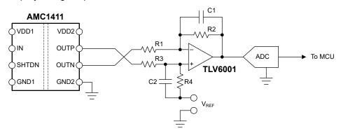
Figure 8-3. Connecting the AMC1411 Output to a Single-Ended Input ADC
