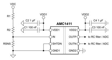
Figure 9-1. Decoupling of the AMC1411
