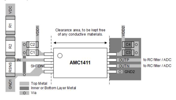
Figure 10-1. Recommended Layout of the AMC1411
