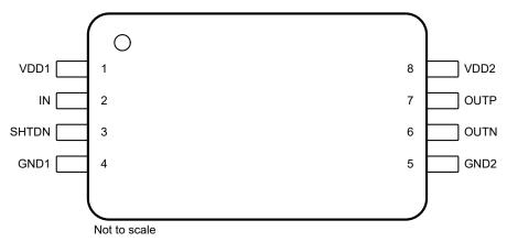
Figure 5-1. DWL Package, 8-Pin SOIC (Top View)
