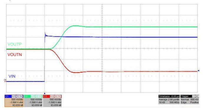
Figure 8-4. Step Response of the AMC1411
