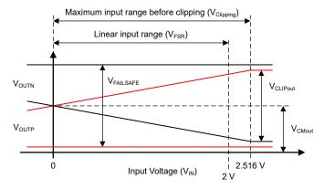
Figure 7-2. Output Behavior of the AMC1411
