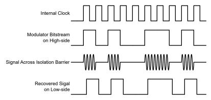
Figure 7-1. OOK-Based Modulation Scheme
