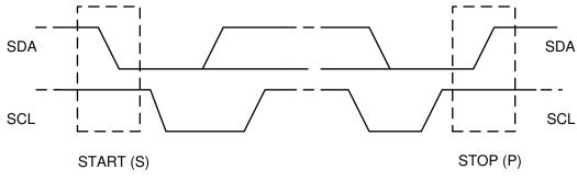
Figure 8-14. START and STOP Conditions on the I<sup>2</sup>C Bus
