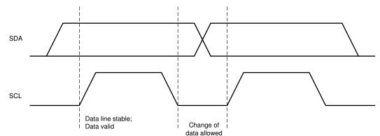
Figure 8-13. Bit Transfers on the I<sup>2</sup>C Bus
