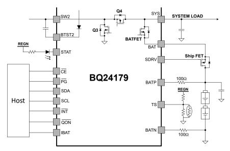
Figure 8-12. The Application Diagram for the External Ship FET
