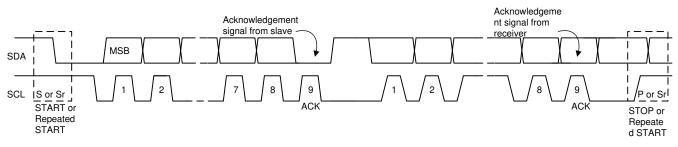
Figure 8-15. Data Transfer on the I<sup>2</sup>C Bus
