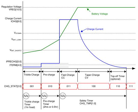
Figure 8-8. Battery Charging Profile
