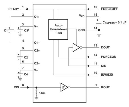
$<sup>^{\</sup>dagger}$  C3 can be connected to  $V_{CC}$  or GND.
