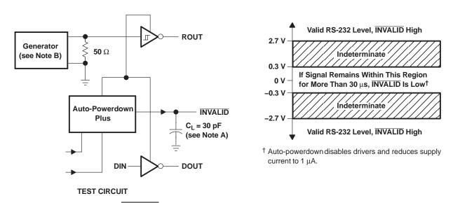
Figure 4. INVALID Propagation Delay Times and Driver Enabling Time
