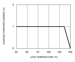
Fig.1 Forward Current Derating Curve
