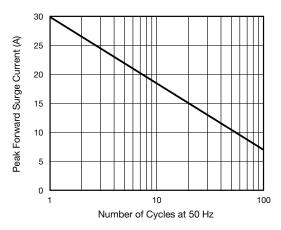
Fig. 3 - Max. Non-Repetitive Peak Forward Surge Current
