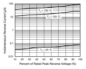
Fig. 5 - Typical Reverse Leakage Characteristics
