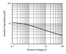
Fig. 6 - Typical Junction Capacitance
