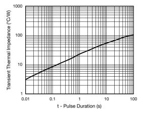
Fig. 7 - Typical Transient Thermal Impedance
