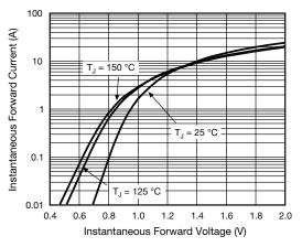
Fig. 4 - Typical Instantaneous Forward Characteristics
