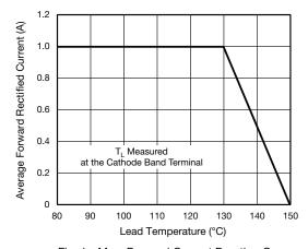
Fig. 1 - Max. Forward Current Derating Curve
