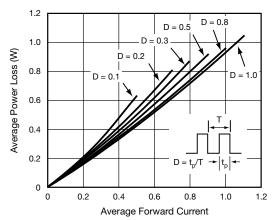
Fig. 2 - Forward Power Loss Characteristics
