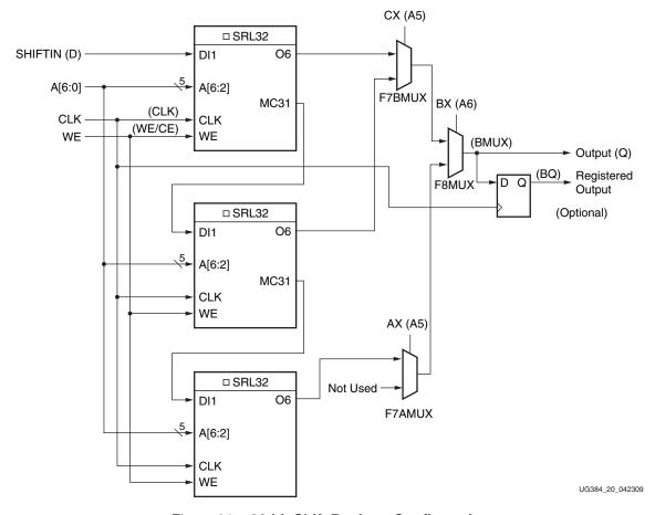
Figure 21: 96-bit Shift Register Configuration
