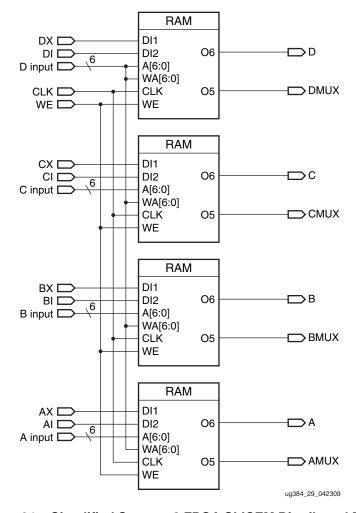
Figure 34: Simplified Spartan-6 FPGA SLICEM Distributed RAM
