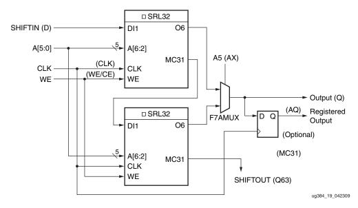
Figure 20: 64-bit Shift Register Configuration
