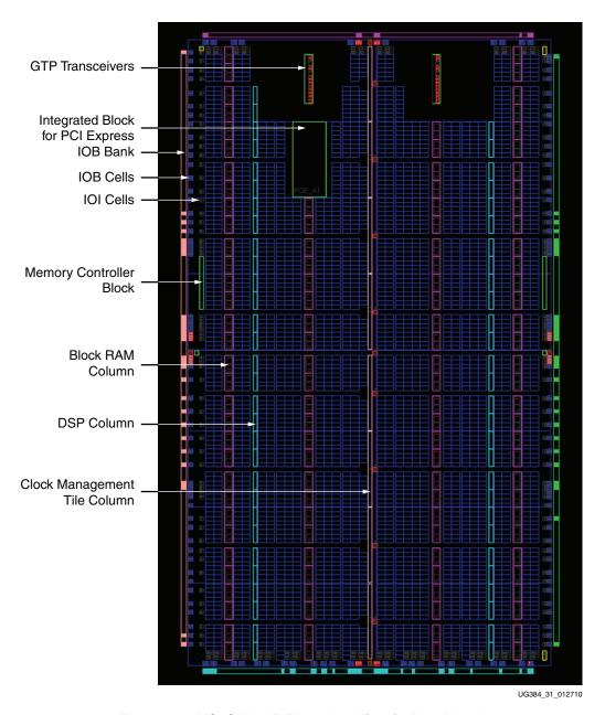
Figure 31: XC6SLX45T Floorplan View in PlanAhead
