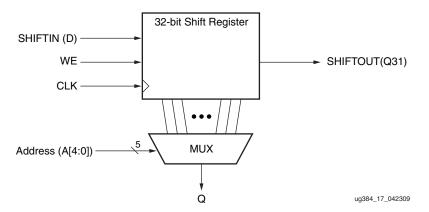
Figure 18: Representation of a Shift Register
