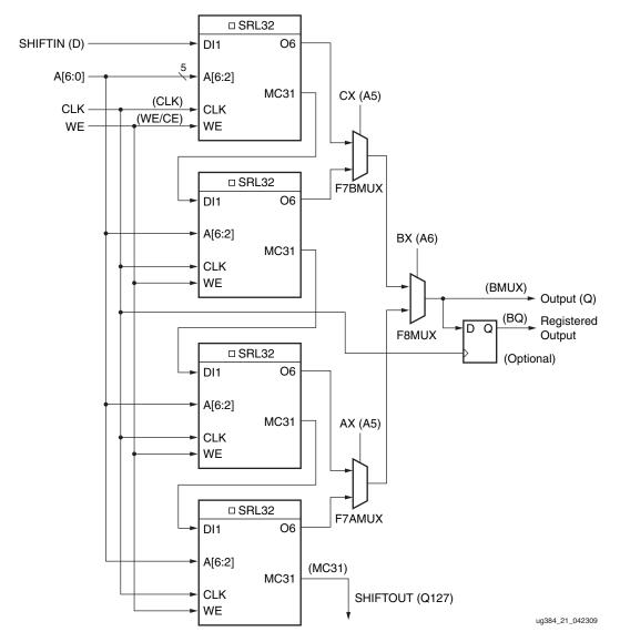
Figure 22: 128-bit Shift Register Configuration
