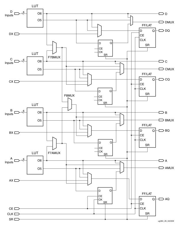
Figure 32: Simplified Spartan-6 FPGA Slice
