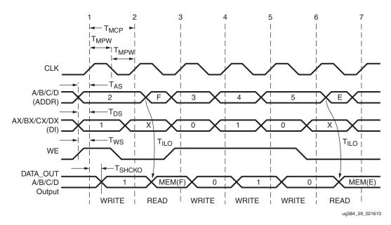
Figure 35: Slice Distributed RAM Timing Characteristics
