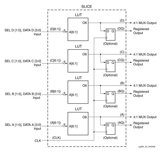
Figure 23: Four 4:1 Multiplexers in a Slice
