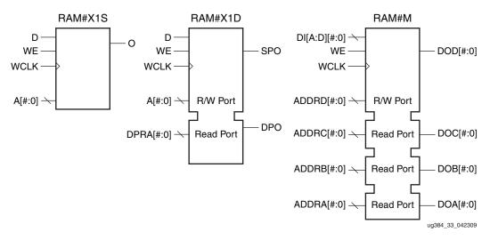
Figure 39: Single-Port, Dual-Port, and Quad-Port Distributed RAM Primitives
