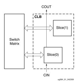
Figure 1: Arrangement of Slices within the CLB
