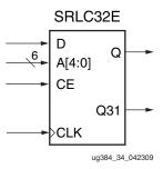
Figure 40: 32-bit Shift Register
