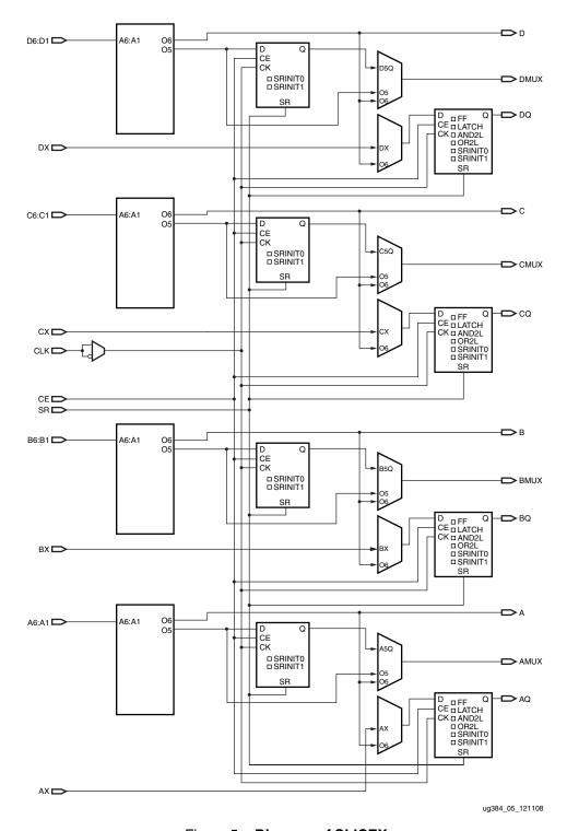
Figure 5: Diagram of SLICEX
