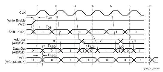
Figure 37: Slice SRL Timing Characteristics
