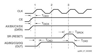
Figure 33: General Slice Timing Characteristics
