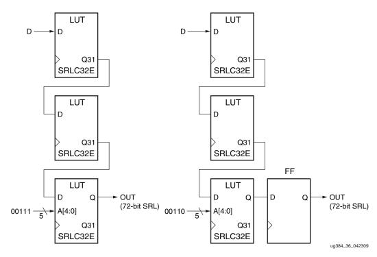
Figure 42: Example Static-Length Shift Register
