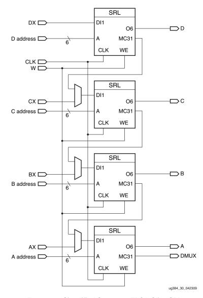
Figure 36: Simplified Spartan-6 FPGA Slice SRL
