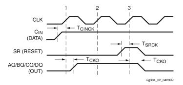
Figure 38: Slice Carry-Chain Timing Characteristics
