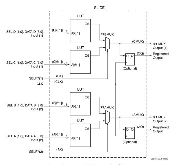
Figure 24: Two 8:1 Multiplexers in a Slice
