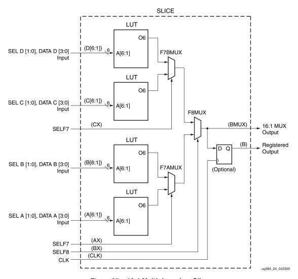
Figure 25: 16:1 Multiplexer in a Slice
