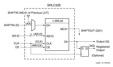
Figure 17: 32-bit Shift Register Configuration
