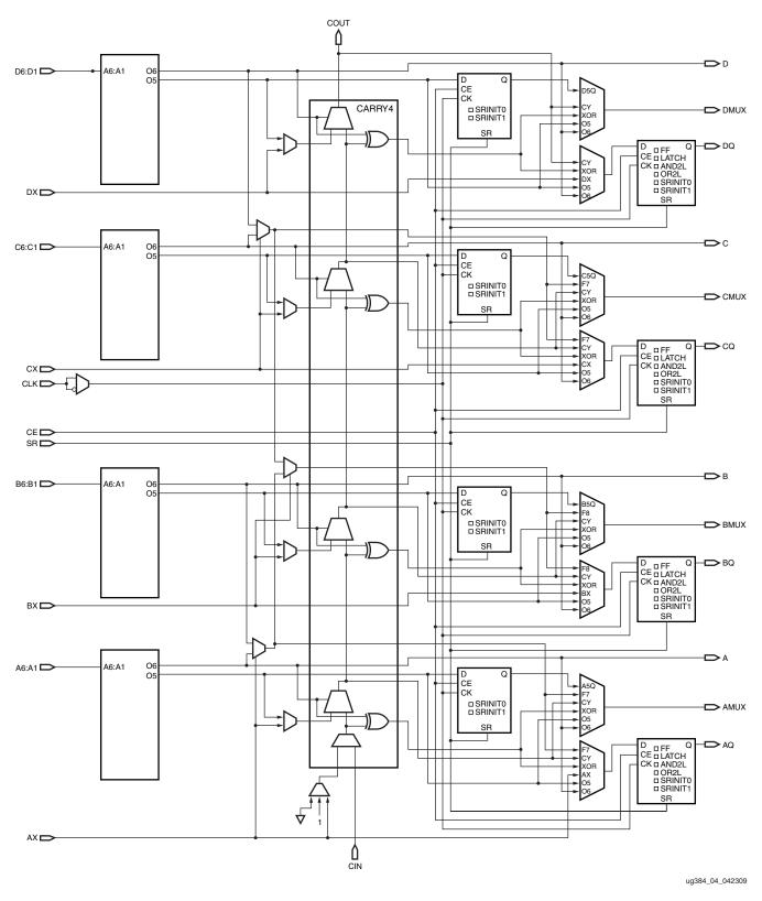
Figure 4: Diagram of SLICEL
