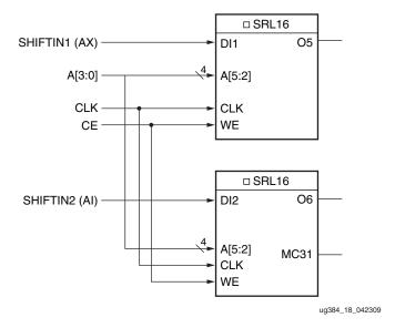
Figure 19: Dual 16-bit Shift Register Configuration
