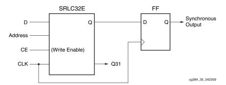
Figure 41: Synchronous Shift Register
