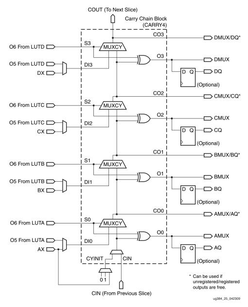
Figure 26: Fast Carry Logic Path and Associated Elements
