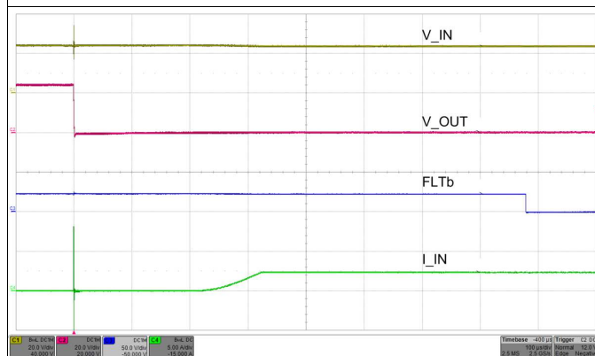
Figure 27. OVP Overvoltage Cut-Off Response
