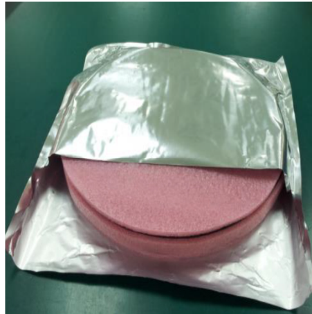
Vacuum-Sealed Moisture Barrier Bag with inner foam lining, MSL3, Caution, and Barcode Labels
