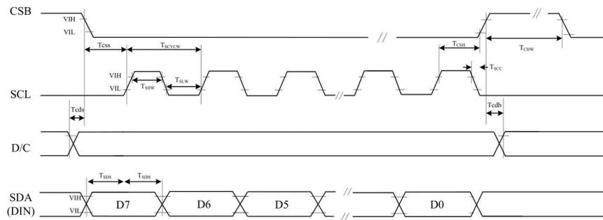
4 pin serial interface characteristics
