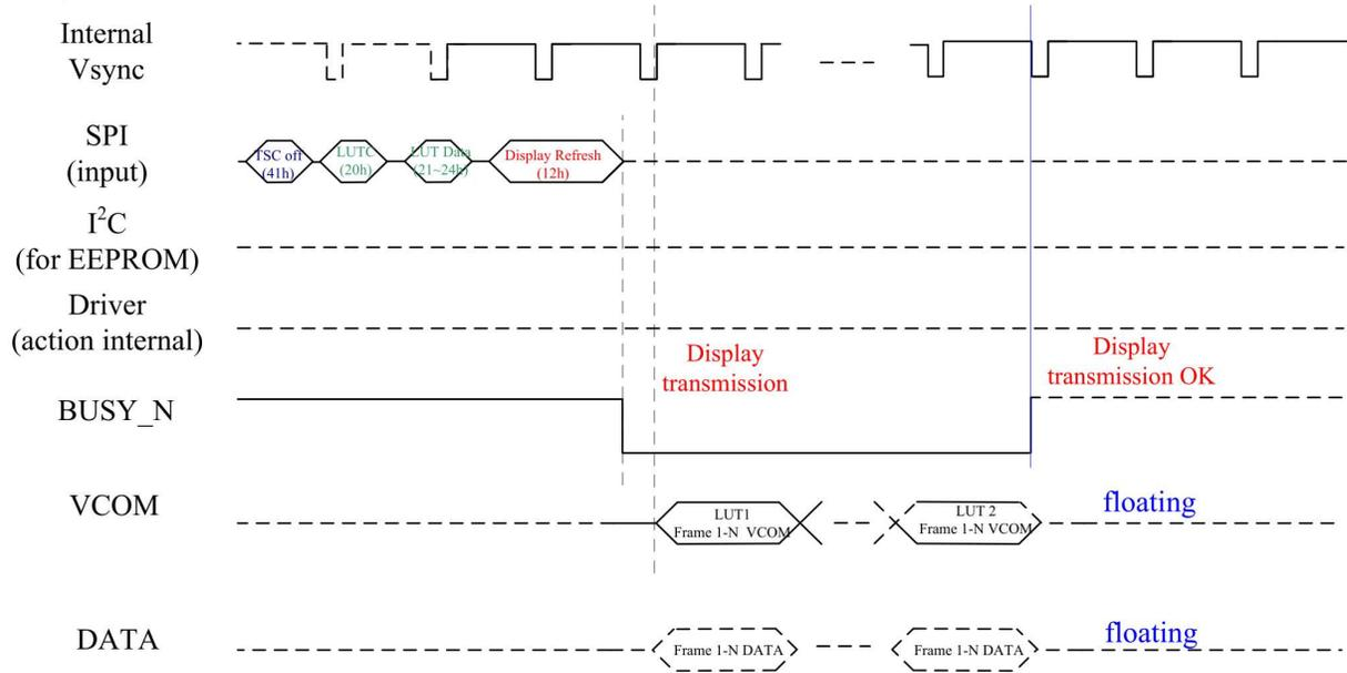
Figure 6: Display refresh example2 waveform
