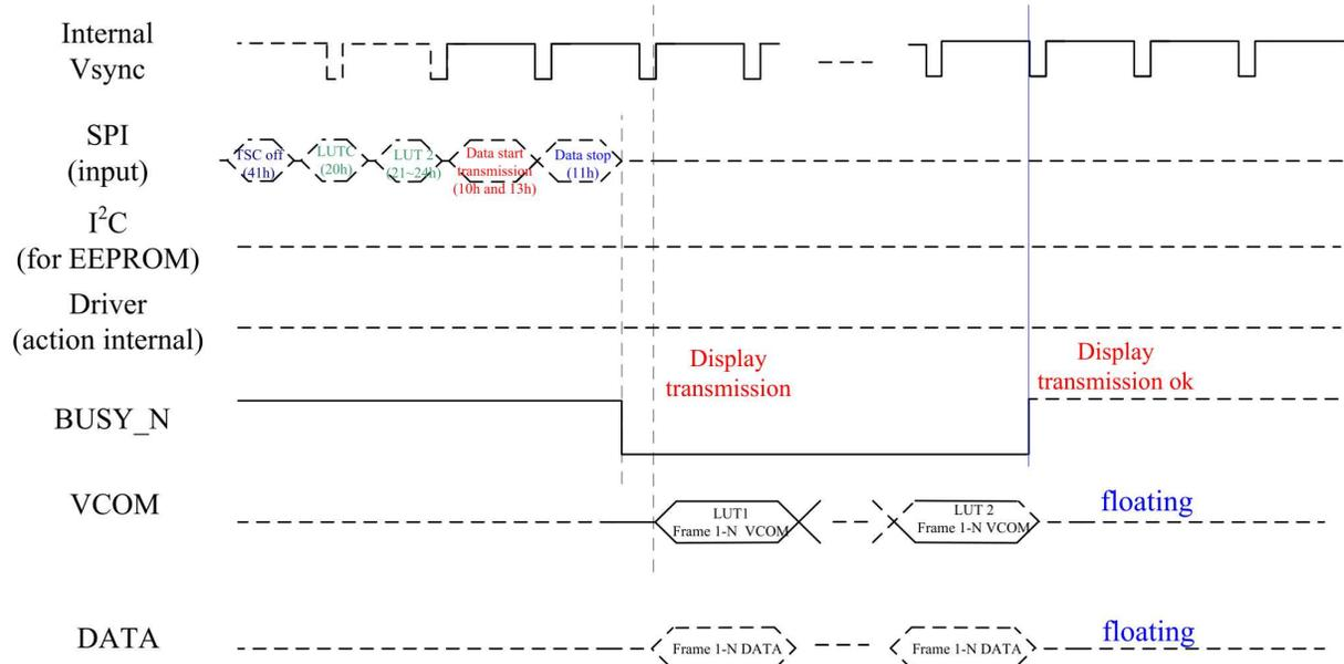
Figure 4: Data transmission example 2 waveform
