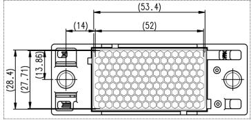
Dimension in mm, tolerance: ±1 mm
