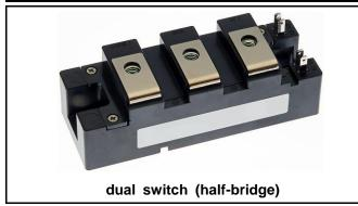
Collector current Ic ..... 150A Collector-emitter voltage VCES ..... 6 5 0 V Maximum junction temperature T<sub>vimax</sub> ...... 175°C dual switch (half-bridge) •Copper base plate (Nickel-plating) Nickel-plating tab terminals • RoHS Directive compliant
