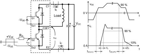
Switching characteristics test circuit and waveforms
