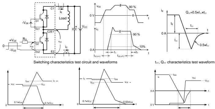
IGBT Turn-off switching energy Turn-on / Turn-off switching energy and Reverse recovery energy test waveforms (Integral time instruction drawing)
