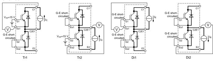
V<sub>CEsat</sub> characteristics test circuit
