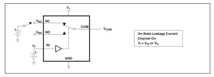
Figure 17. On-State Leakage Current ( $I_{COM(ON)}$ ,  $I_{NC(ON)}$ ,  $I_{NO(ON)}$ )
