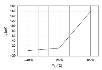
Figure 14. Power-Supply Current vs Temperature  $(V_+ = 5 V)$
