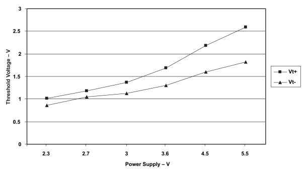
Figure 1. Logic Threshold vs Power Supply
