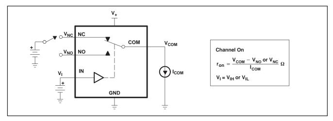
Figure 15. On-State Resistance (r<sub>on</sub>)
