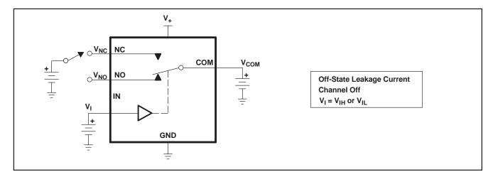
$\textbf{Figure 16. OFF-State Leakage Current (I_{NC(OFF)}, I_{NC(PWROFF)}, I_{NO(OFF)}, I_{NO(PWROFF)}, I_{COM(OFF)}, I_{COM(PWROFF)})}$
