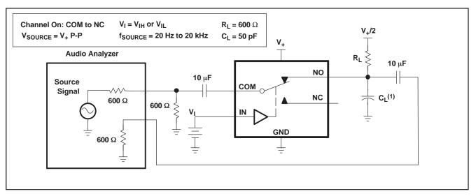
A. C<sub>L</sub> includes probe and jig capacitance.
