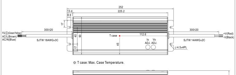
X IP65 rated. Output voltage and constant current level can be adjusted through internal potentiometer. (Can access by removing the rubber stopper on the case.)
