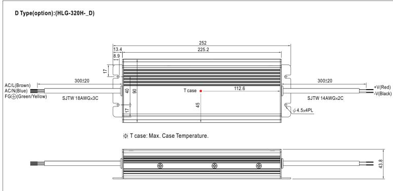
X IP67 rated. Timer dimming function, contact MEAN WELL for details.
