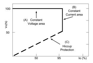
Typical LED power supply I-V curve
