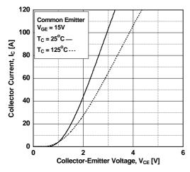
Figure 5. Saturation Voltage vs. Case
