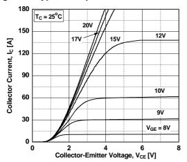
Figure 3. Typical Saturation Voltage Characteristics
