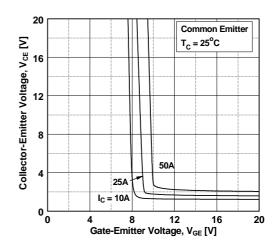
Figure 7. Saturation Voltage vs. V<sub>GE</sub>
