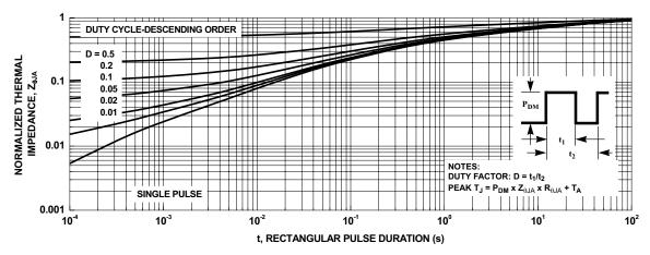
Figure 11. Transient Thermal Response Curve
