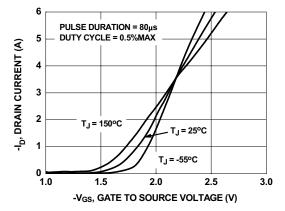
Figure 5. Transfer Characteristics
