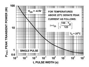
Figure 10. Single Pulse Maximum Power Dissipation
