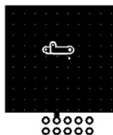
a. 53\text{ }^\circ\text{C/W} when mounted on a 1\text{ in}^2 pad of 2 oz copper
