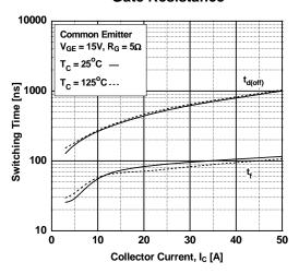
Figure 16. Turn-off Characteristics vs.
