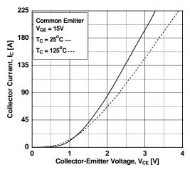
Figure 5. Saturation Voltage vs. Case
