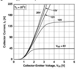
Figure 3. Typical Saturation Voltage Characteristics
