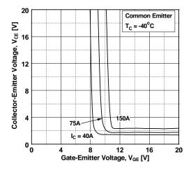
Figure 7. Saturation Voltage vs. V<sub>GE</sub>
