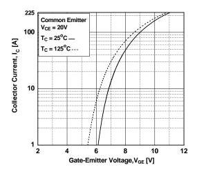
Figure 6. Saturation Voltage vs. V<sub>GE</sub>
