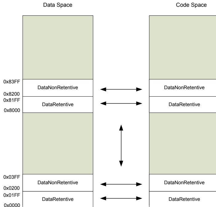
Figure 37. Configurability of SRAM address space location
