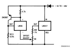
FIGURE 9. 4-To-20 mA Current Source (0°C to +100°C)
