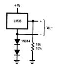
FIGURE 7. Temperature Sensor, Single Supply, -55° to +150°C
