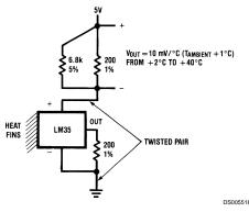
FIGURE 5. Two-Wire Remote Temperature Sensor (Grounded Sensor)
